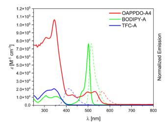
Fig. 3 UV/Vis (solid line) and fluorescence (dashed line) spectra of OAPPDO-A4, BODIPY-A, and TFC-A measured in CHCl<sub>3</sub>. Excitation wavelength for the emission spectra for the respective compound OAPPDO-A4 (531 nm), BODIPY-A (502 nm), and TFC-A (344 nm) ( $c \approx 10^{-5}$  M).
