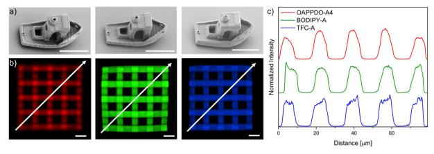
Fig. 5 (a) The benchmarking structures consisting of boats were fabricated out of the same formulation as the lattice below and imaged via SEM (Scalebars = 10 µm). (b) 2PLP printed lattices with the red, green, and blue formulation, which were imaged via confocal microscopy. (c) The intensity of the respective lattice was plotted along the white arrow against the distance.
