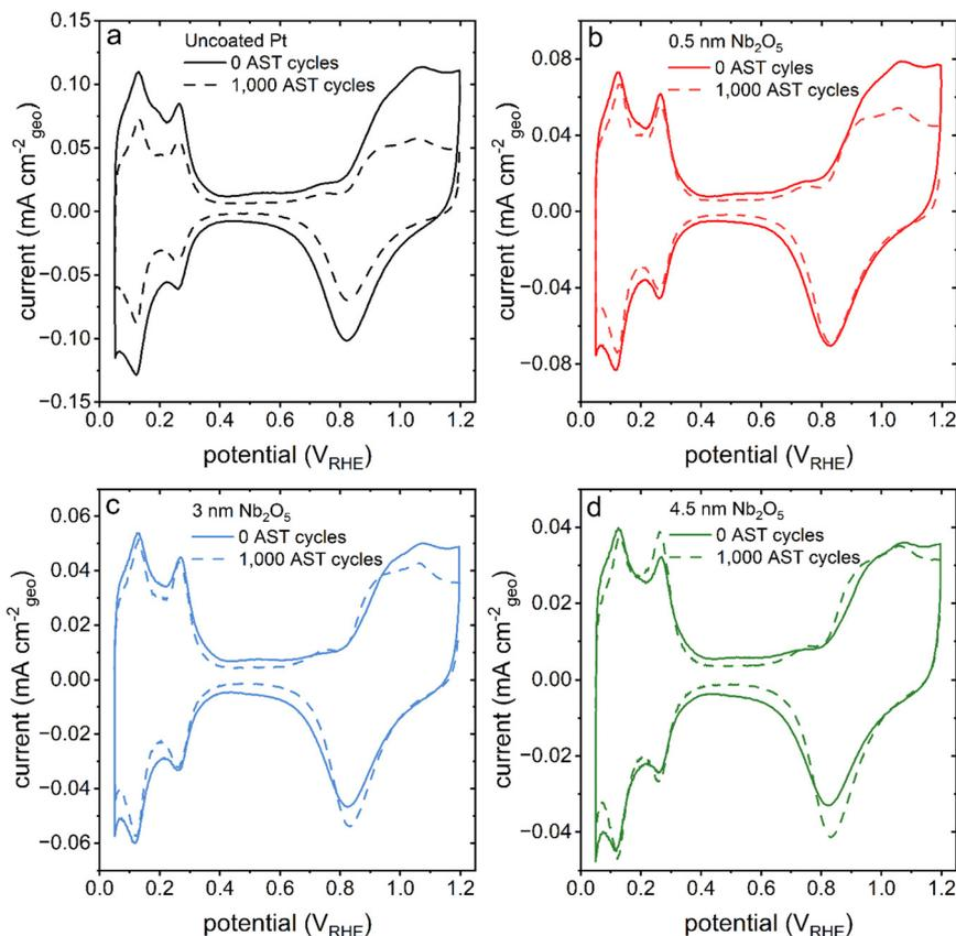
**Fig. 6** A series of cyclic voltammograms corresponding to the nanotextured Pt catalysts (solid line) before and (dashed line) after 1000 cycles of an accelerated stress test (AST). The colours of the traces correlate to differences in thickness of the  $\text{Nb}_2\text{O}_5$  coatings, where (a) black represents uncoated or pristine nanotextured Pt, and (b) red is 0.5 nm, (c) blue is 3 nm, and (d) green is 4.5 nm thick niobia coated nanotextured Pt.
