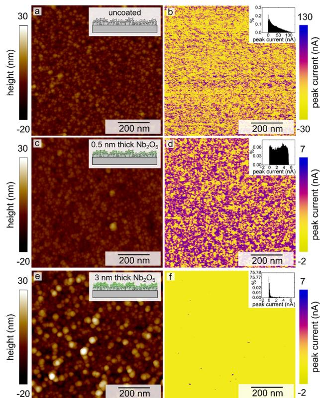
**Fig. 3** Conductive atomic force microscopy images displaying the measured sample height (a, c and e) and peak current (b, d and f) for a pristine, uncoated electrodeposited Pt catalyst (a and b), and these nanotextured Pt catalysts after coating with a 0.5 nm (c and d) and a 3 nm thick layer of  $\text{Nb}_2\text{O}_5$  (e and f). Histograms of the measured peak currents are plotted as insets to each, corresponding CAFM map.
