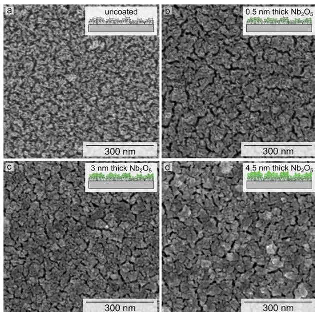
**Fig. 5** A series of scanning electron microscopy (SEM) images of (a) pristine Pt with a nanoscale texture and the same substrate after coating with a (b) 0.5 nm, (c) 3 nm, and (d) 4.5 nm thick layer of Nb<sub>2</sub>O<sub>5</sub>. These images were taken after 1000 cycles of an AST.
