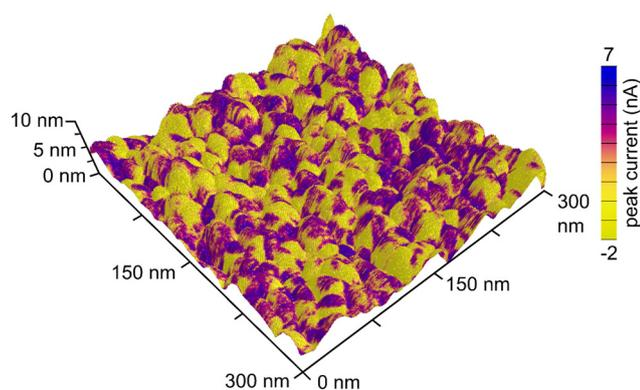
**Fig. 2** Three-dimensional image of the topography of electrodeposited Pt coated with a 0.5 nm thick layer of  $\text{Nb}_2\text{O}_5$ . The topography is overlaid with an electrical conductivity map (e.g., peak current values) as measured by conductive atomic force microscopy (C-AFM).
