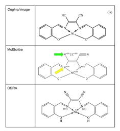
Fig. 8 A common transition metal complex Ia from US-7001437-B2 above and MolScribe's prediction below. For MolScribe – green arrow: isonitrile group instead of nitrile group, yellow arrow: wrongly predicted valency of 4 at the nitrogen atoms participating in a dative bond. In contrast, OSRA is interpreting the dative bonds between the nitrogen atoms and nickel correctly but the ionic bonds between the oxygens and the metal are not understood.
