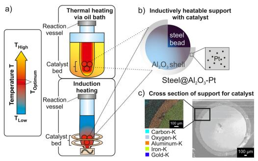
Fig. 1 a) Scheme of heat input into a fixed-bed reactor via inductive (on the bottom) versus thermal heating (on the top). b) Scheme of the synthesized  $Steel@Al_2O_3$ —Pt catalyst particle consisting of a steel core and an alumina shell impregnated with Pt. c) SEM image of a cross-section of the Steel@Al<sub>2</sub>O<sub>3</sub>-Pt and its elemental mapping via energy-dispersive X-ray spectroscopy.
