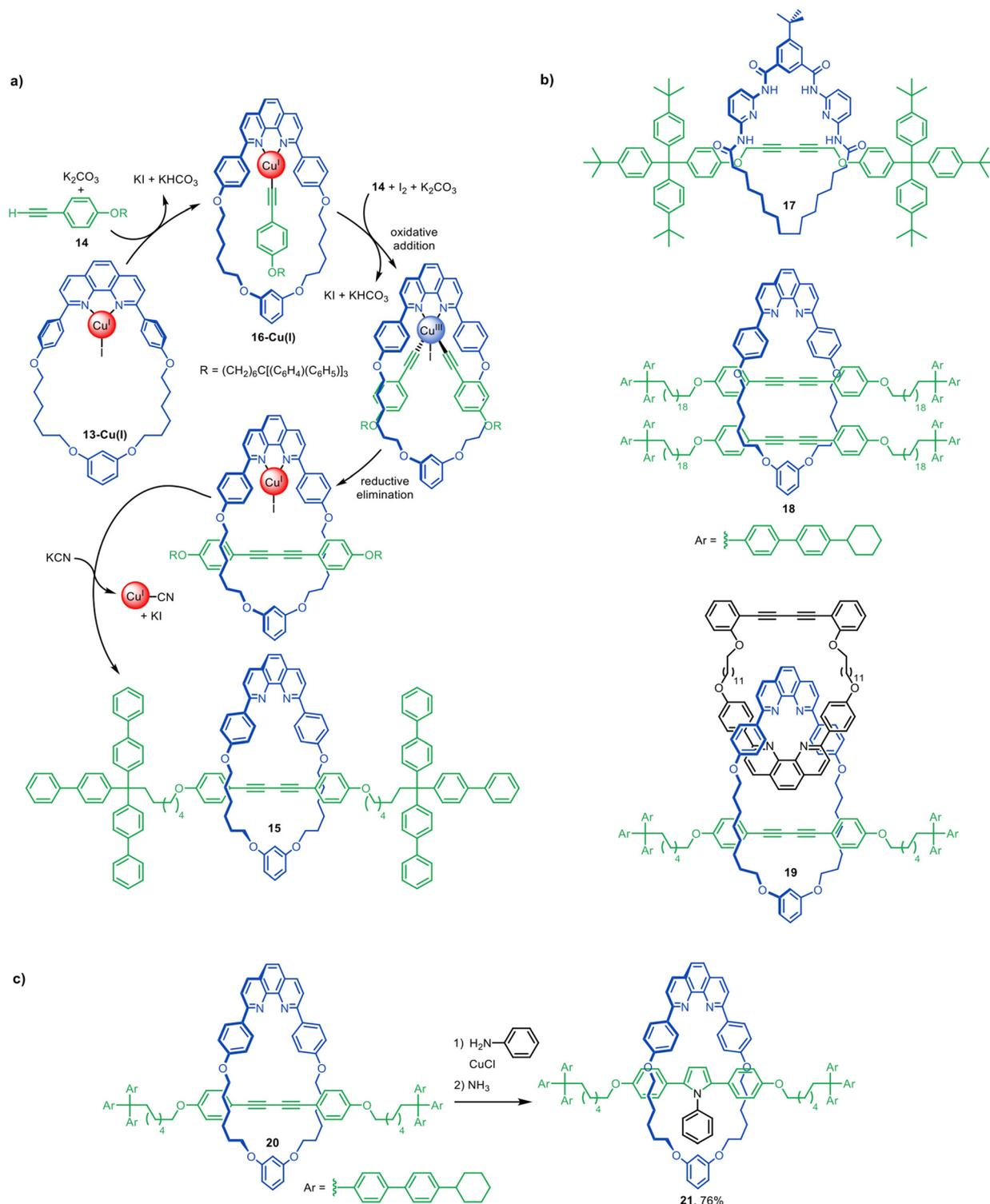
**Fig. 6** (a) Proposed mechanism for the active template synthesis of [2]rotaxanes through the Cu(I)-mediated Glaser–Hay homocoupling of terminal alkynes.<sup>46</sup> (b) Selected examples of interlocked structures synthesised by active template Glaser couplings.<sup>47–49</sup> (c) Saito's post-assembly modification of a diyne rotaxane to an aryl pyrrole rotaxane.<sup>50</sup>
