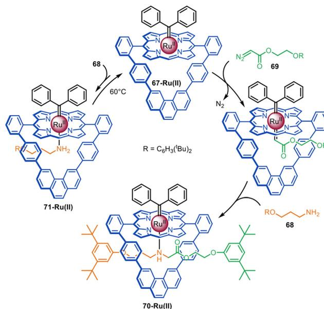
Fig. 20 Megiatto’s active template synthesis of [2]rotaxanes via Ru(II)-mediated N–H carbene insertion.<sup>116</sup>
