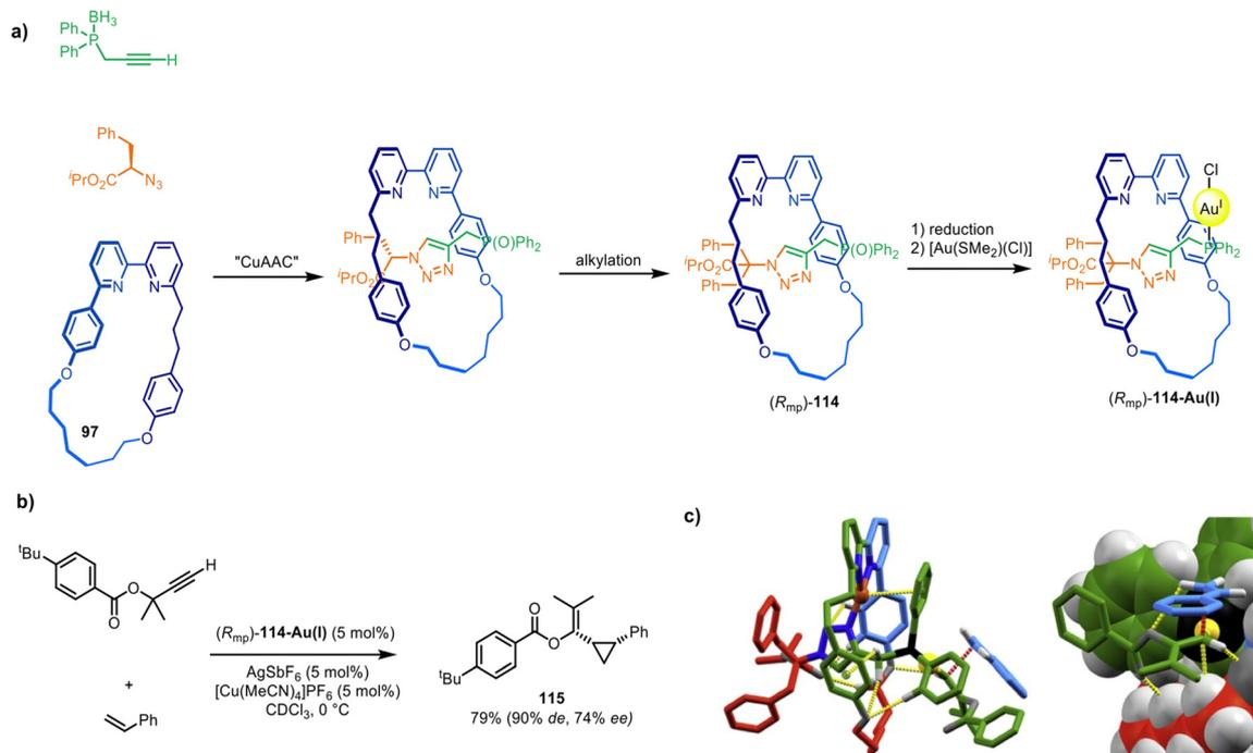
Fig. 37 (a) Goldup's active template synthesis of mechanically planar chiral rotaxane precatalyst  $(R_{mp})$ -114-Au(I). (b) Example of a diastereoselective and enantioselective Toste-Ohe-Uemura cyclopropanation reaction promoted by **114-Au(I)**. (c) Computationally modelled transition state.<sup>166</sup>
