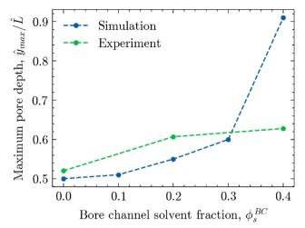
Fig. 9 The maximum pore depth  $\hat{y}_{\text{max}}/\hat{L}$ , corresponding to the relative depth within the bijel cross-section where the pore size reaches its maximum value, *versus* the solvent fraction of the interior bore channel  $\phi_s^{BC}$ . The green markers correspond to experimental bijel structures, whereas the blue markers correspond to the structures provided by the phase-field model.
