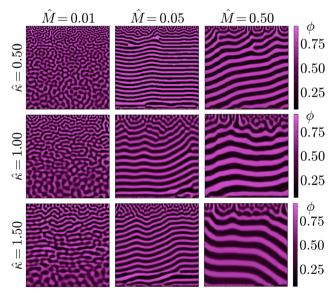
Fig. 4 Final morphologies of the phase-separated oil/water mixtures after STrIPS for different values of the relative mobility  $\hat{M}$  and the gradient energy coefficient  $\hat{\kappa}$ . Lower values of  $\hat{M}$  and  $\hat{\kappa}$  yield relatively isotropic phase separation, whereas higher values result in laminar structures with a more isotropic surface region.
