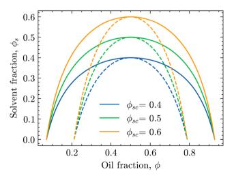
Fig. 1 Phase diagrams of the oil/water mixture with respect to the solvent volume fraction  $\phi_{\rm s}$  for different values of  $\phi_{\rm sc}.$  The solid and dashed lines are the binodal and spinodal curves, respectively, calculated using eqn (4) and (6) for  $\chi_0 = 3.0$ .
