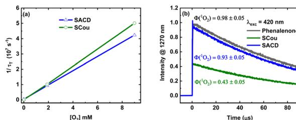
**Fig. 10** (a) Determination of the bimolecular triplet quenching constants of SAcD and SCoU by molecular oxygen. Inverse triplet lifetime vs. concentration of molecular oxygen in acetonitrile. (b) Phosphorescence decay traces for singlet oxygen monitored at 1270 nm generated by pulsed photoexcitation at 420 nm of SAcD, SCoU, or Phenalenone in air-saturated acetonitrile solutions.
