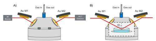
Fig. 2 Schematic of the Teflon cell used for IRRAS experiments of NO<sub>2</sub> flowing over the PC surface. Panel A depicts the outside of the Teflon cell with the IR beam from the spectrometer being directed into the cell through the ZnSe windows. In panel B, the inside of the cell is shown and includes the IR beam reflecting off the PC interface within the Petri dish.
