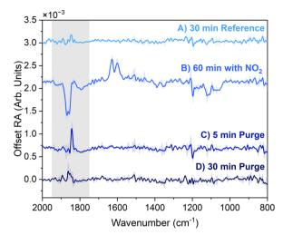
Fig. 4 IRRAS spectra of the surface of PC before, during, and after exposure to 5.1 ppm NO2. (A) 30 min reference (B) 60 min with NO2 (C) 5 min of purging NO<sub>2</sub> with N<sub>2</sub> and air. (D) 30 min of purging NO<sub>2</sub> with N<sub>2</sub> and air. Spectra plotted are an average of two trials and the standard deviation is plotted as shading. Spectra are offset for clarity and the carbonyl region (1950–1750 cm<sup>-1</sup>) is highlighted with grey shading.
