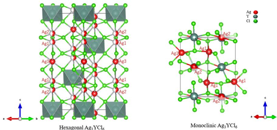
Fig. 3 Crystal structure models of hexagonal and monoclinic  $\text{Ag}_3\text{YCl}_6$ . In the monoclinic phase, the Ag occupancy of Ag1 and Ag2 sites is 0.5. The crystal structure of the monoclinic phase was optimized by atomic simulation at 0 GPa and was drawn using VESTA.<sup>18</sup>
