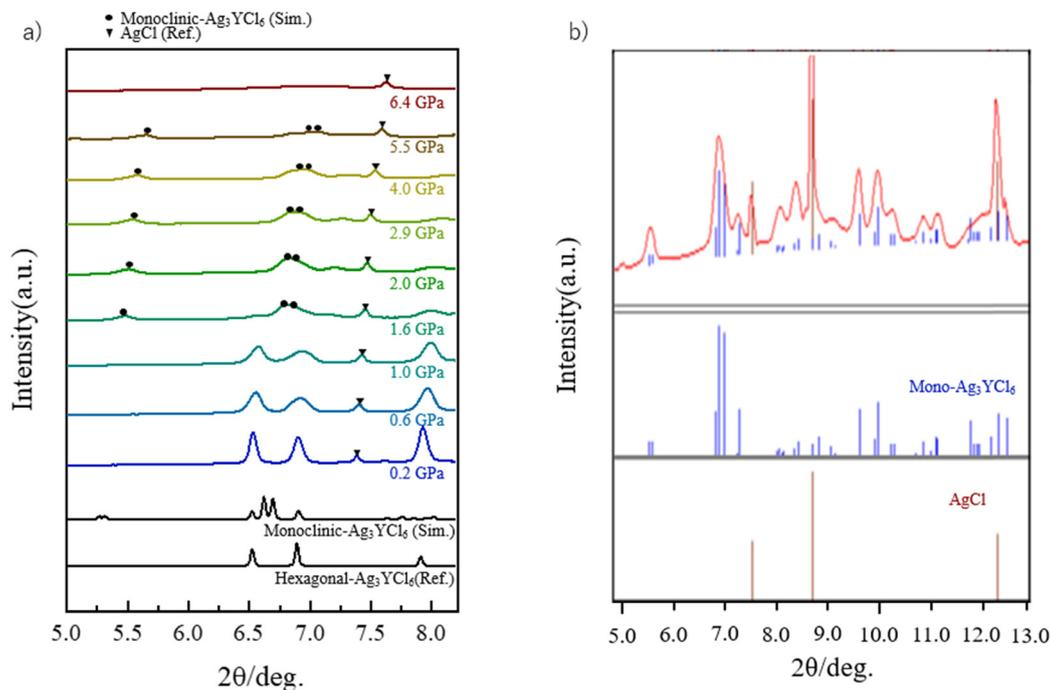
Fig. 1 Phase transition of hexagonal  $\text{Ag}_3\text{YCl}_6$  under pressure. a) *In situ* XRD patterns of  $\text{Ag}_3\text{YCl}_6$  under hydrostatic pressure ( $\lambda = 0.412739$  Å). b) Comparison of the XRD pattern of hexagonal  $\text{Ag}_3\text{YCl}_6$  under 2.0 GPa and the simulated pattern of monoclinic  $\text{Ag}_3\text{YCl}_6$ .<sup>18</sup>
