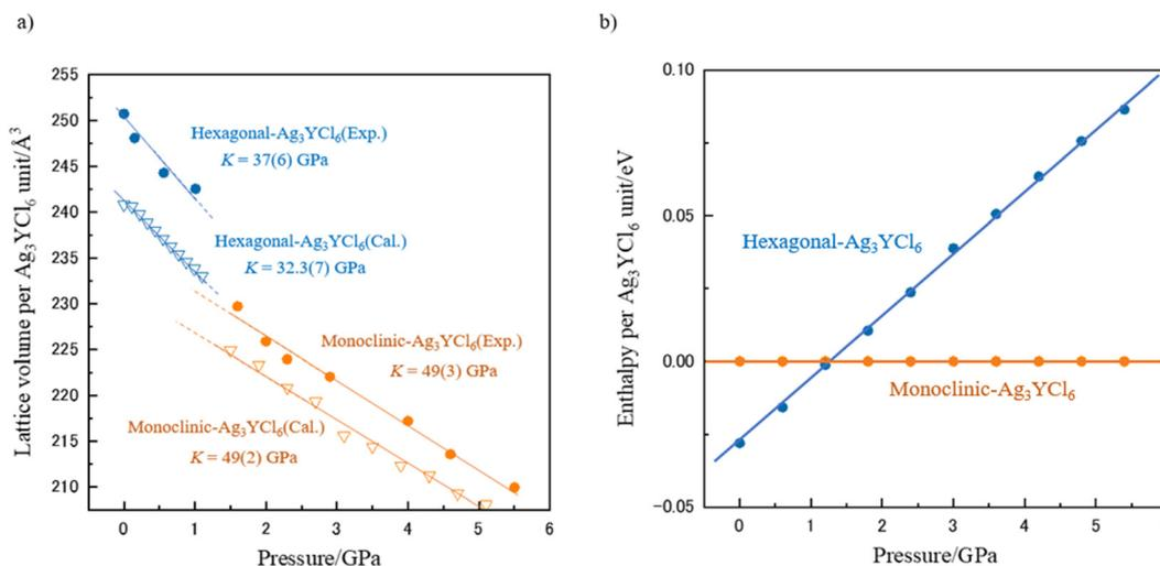
Fig. 2 a) Pressure-dependent lattice volumes of hexagonal  $\text{Ag}_3\text{YCl}_6$  and monoclinic  $\text{Ag}_3\text{YCl}_6$  (experiment: circle, simulation: triangle). b) Pressure-dependent calculated enthalpy of hexagonal  $\text{Ag}_3\text{YCl}_6$  relative to the monoclinic phase.
