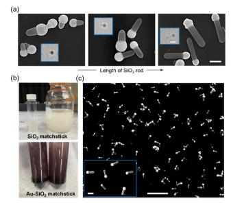
Fig. 4 (a) SEM images of the Au-SiO<sub>2</sub> Janus matchsticks with a tunable aspect ratio. Insets are the corresponding microscope images of SiO<sub>2</sub> Janus matchsticks before gold coating. Scale bars =  $1 \mu m$ . (b) Pictures showing the ability to increase the reaction volume and produce Au-SiO<sub>2</sub> Janus matchsticks in gram scale. (c) A zoom-out SEM image of Au-SiO<sub>2</sub> Janus matchsticks. Scale bar = 10  $\mu$ m. Inset is the zoom-in image. Scale bar = 1  $\mu$ m.
