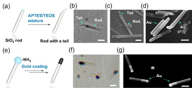
**Fig. 3** (a)–(c) Schematic, optical microscope and SEM images showing that adding APTES and TEOS as a mixture forms a silica tail at the end of rod. (d) SEM image shows that rods are coated with gold. (e) Schematic illustration showing gold coating on matchsticks in the absence of TEOS addition. (f)–(g) Optical microscope and SEM images show that gold is selectively coated at the tip of the rods where water droplets were attached to. Scale bars = 1  $\mu\text{m}$ .
