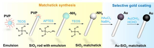
Fig. 1 Schematic showing the synthesis of SiO<sub>2</sub> matchstick with an amine-functionalized head and the site-specific gold coating to form Au–SiO<sub>2</sub> matchstick.
