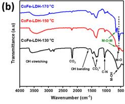
Fig. 2 FT-IR spectra of (a) pristine CoFe-LDH and CoFe-LDH@NGF, and (b) samples prepared at different temperatures (i.e. 130, 150 and 170 °C).
