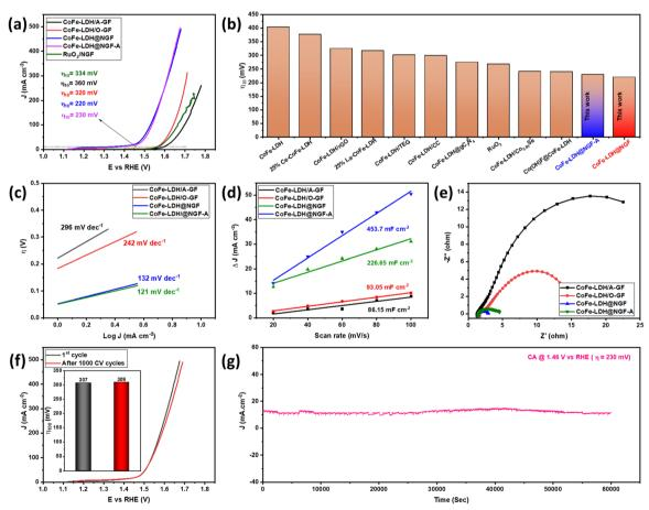
Fig. 4 iR-corrected polarization curves (a), comparison of CoFe-LDH@NGF with literature reports (b), comparison of Tafel plots (c), double layer capacitance ( $C_{cl}$ ) at different scan rates (d), and EIS Nyquist spectra (e) of CoFe-LDH@A-GF, CoFe-LDH@O-GF, CoFe-LDH@NGF and CoFe-LDH@NGF-A in 1.0 M KOH. Comparison of LSV curves (f) and  $\eta_{100}$  (inset) before and after 1000 CV cycles (g). Chronoamperometry analysis performed at overpotential of 230 mV.
