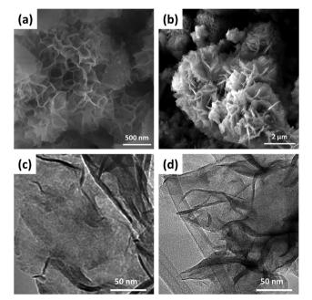
Fig. 5 Comparison of SEM images before (a) and after (b) the OER stability test. TEM images of CoFe-LDH nanosheets before (c) and after (d) chronoamperometry analysis
