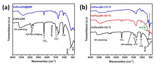
Fig. 2 FT-IR spectra of (a) pristine CoFe-LDH and CoFe-LDH@NGF, and (b) samples prepared at different temperatures (i.e. 130, 150 and 170 °C).
