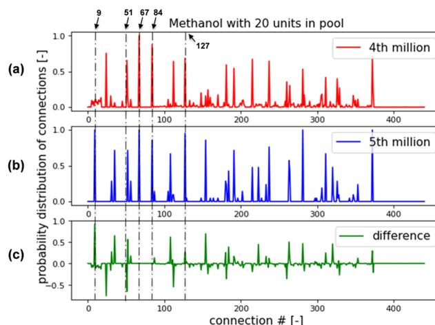
Fig. 17 Probability distribution function of connections for methanol system with 20 units in pool. (a) for feasible flowsheets found within the 4<sup>th</sup> million of episodes; (b) for feasible flowsheets found within the 5<sup>th</sup> million of episodes; (c) Difference between (b) and (a).
