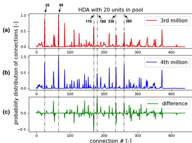
Fig. 16 Probability distribution function of connections for HDA system with 20 units in pool. (a) for feasible flowsheets found within the 3<sup>rd</sup> million of episodes; (b) for feasible flowsheets found within the 4<sup>th</sup> million of episodes; (c) Difference between (b) and (a).
