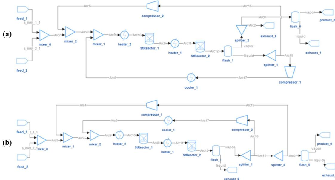
Fig. 11 Optimal flowsheets for HDA system with 20 units in pool. (a) product purity = 99.9%, product flow rate = 0.240 mol s<sup>-1</sup>; (b) product purity = 95.9%, product flow rate = 0.288 mol s<sup>-1</sup>.
