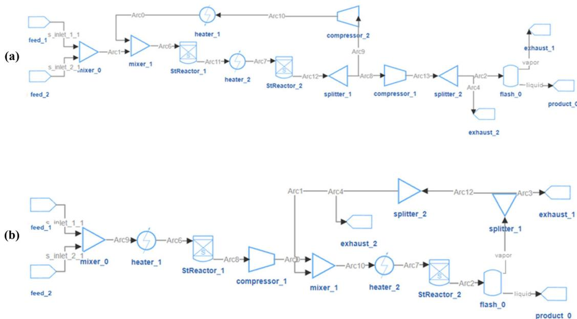
Fig. 14 Optimal flowsheets for methanol system with 18 units in pool. (a) product flow rate =  $0.892 \text{ mol s}^{-1}$ , cost per mole product =  $0.035 \text{ \$ per mol}$ ; (b) product flow rate =  $0.979 \text{ mol s}^{-1}$ , cost per mole product =  $0.051 \text{ \$ per mol}$ .
