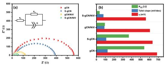
Fig. 6 (a) EIS Nyquist plots and (b) comparison of activity parameters of the studied catalysts.
