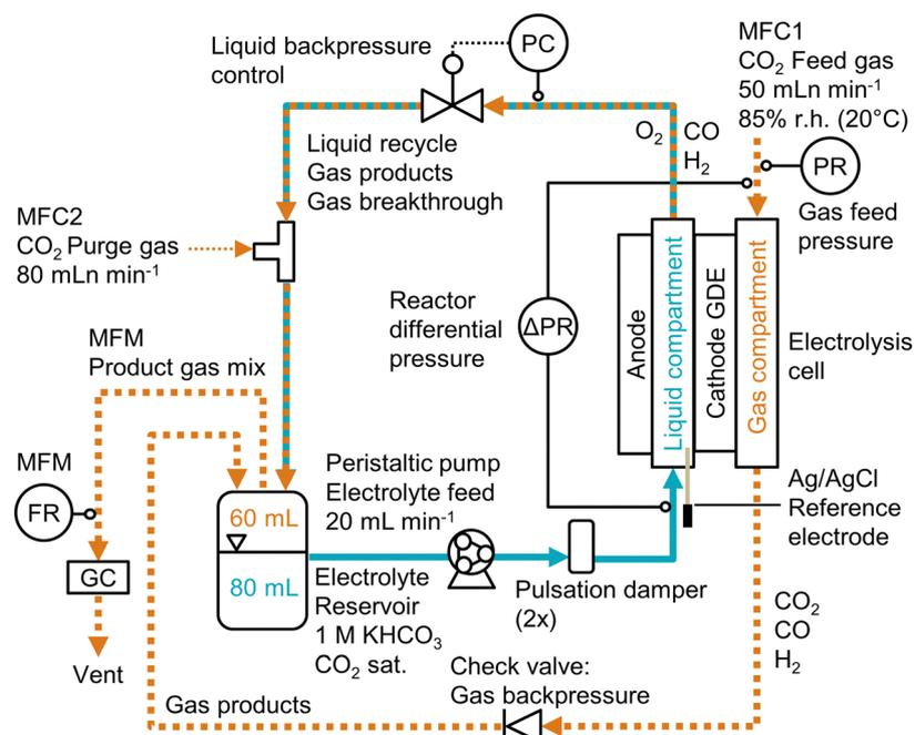
**Fig. 1** Process flow diagram for CO<sub>2</sub> electrolysis setup. The backpressure of the electrolyte stream was controlled (PC) before it was mixed with the purge gas and recirculated. The differential pressure,  $\Delta p$ , across the GDE was measured between the catholyte and gas compartment ( $\Delta\text{PR}$ ). The Faradaic efficiency was determined by recording the product gas flow rate (FR) with a mass flow meter (MFM) and analyzing the gas composition by gas chromatography (GC).
