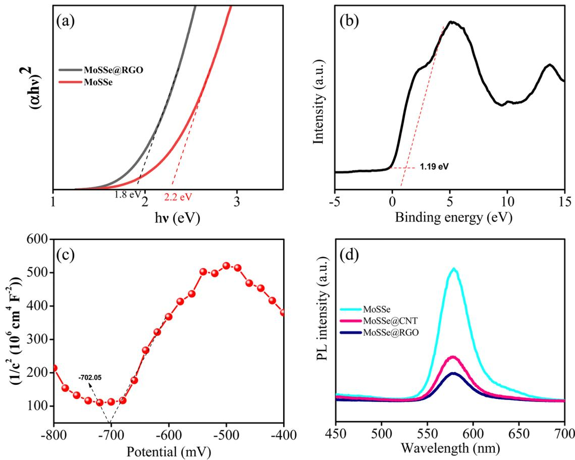
Fig. 7 (a) Tauc plot of MoSSe and the MoSSe@RGO nanocomposite; (b) VB XPS spectra and (c) Mott–Schottky plots of the MoSSe@RGO nanocomposite; (d) PL spectra of an aqueous solution of eosin Y ( $1.0 \times 10^{-7}$  M, excitation wavelength = 490 nm) in the presence of MoSSe@CNT and MoSSe@RGO.
