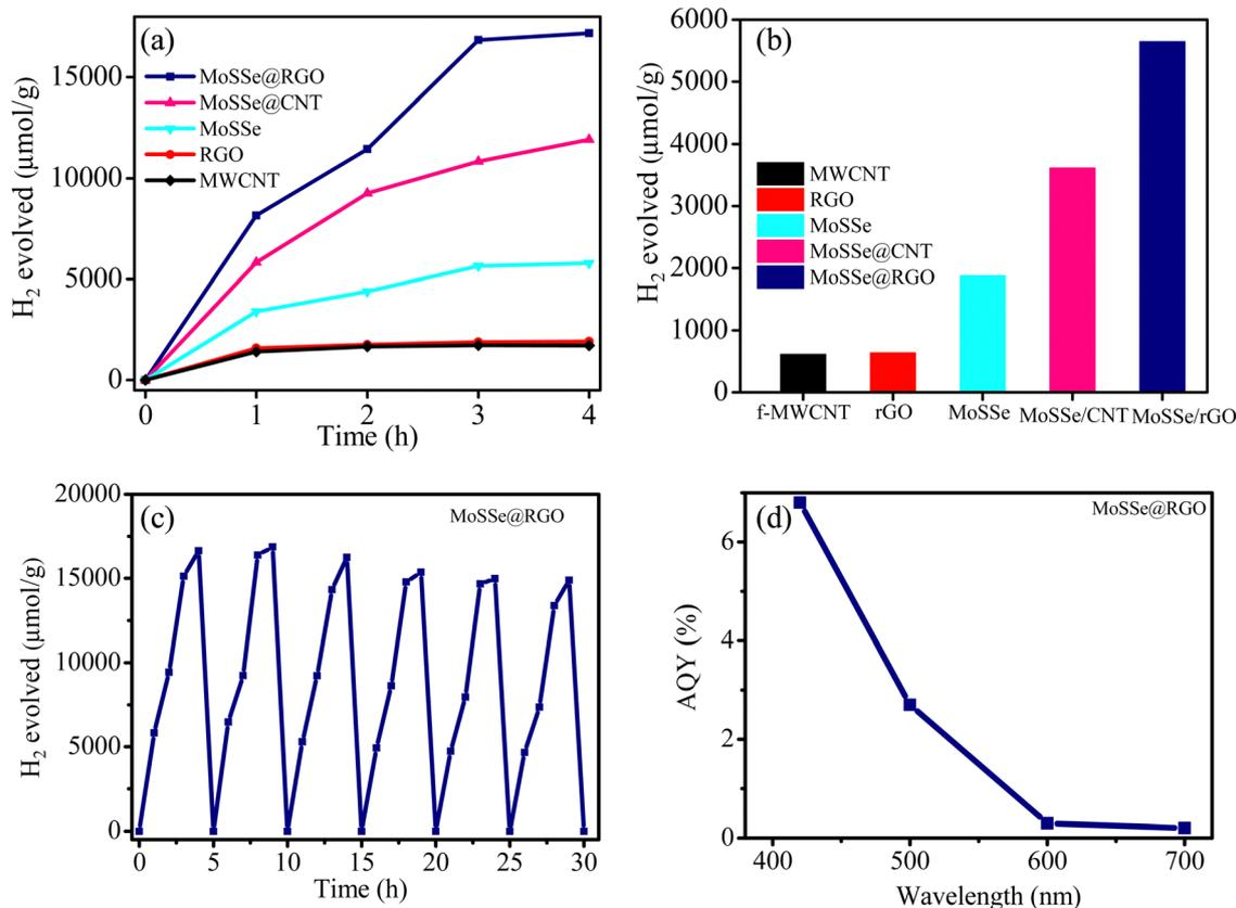
Fig. 6 (a) Photocatalytic H<sub>2</sub> evolution data of the bare MWCNTs, RGO, MoS<sub>2</sub>, MoS<sub>2</sub>@CNT, and MoS<sub>2</sub>@RGO nanocomposites; (b) bar diagram showing the comparison of the HER activities of the samples; (c) cycling stability curve for MoS<sub>2</sub>@RGO nanocomposites and (d) AQY measured on the optimum MoS<sub>2</sub>/RGO catalyst at 420, 500, 600 and 700 nm.
