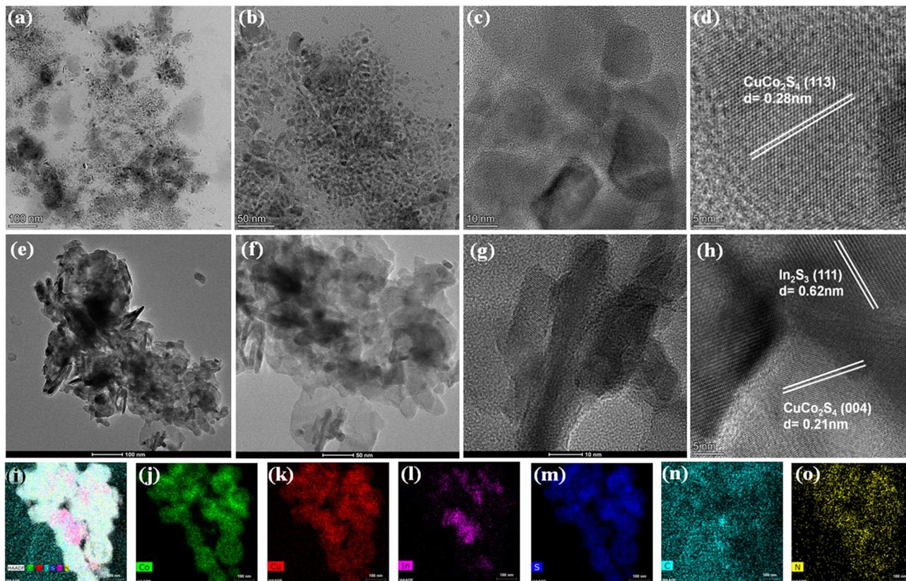
Fig. 2 TEM images of (a) and (b)  $\text{CuCo}_2\text{S}_4$ , and (e) and (f)  $\text{CuCo}_2\text{S}_4/\text{g-C}_3\text{N}_4/\text{In}_2\text{S}_3$ ; HR-TEM images of (c) and (d)  $\text{CuCo}_2\text{S}_4$ , and (g) and (h)  $\text{CuCo}_2\text{S}_4/\text{g-C}_3\text{N}_4/\text{In}_2\text{S}_3$ ; (i)–(o) elemental mapping of Co, Cu, In, S, C, N for  $\text{CuCo}_2\text{S}_4/\text{g-C}_3\text{N}_4/\text{In}_2\text{S}_3$ .
