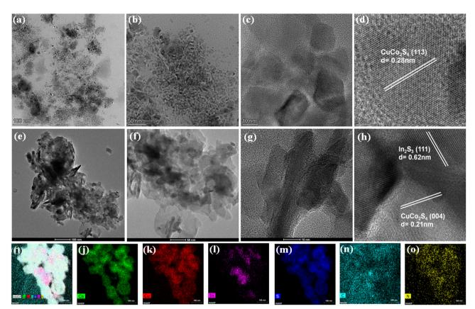
Fig. 2 TEM images of (a) and (b) CuCo<sub>2</sub>S<sub>4</sub>, and (e) and (f) CuCo<sub>2</sub>S<sub>4</sub>/g-C<sub>3</sub>N<sub>4</sub>/In<sub>2</sub>S<sub>3</sub>; HR-TEM images of (c) and (d) CuCo<sub>2</sub>S<sub>4</sub>, and (g) and (h) CuCo<sub>2</sub>S<sub>4</sub>/  $g-C_3N_4/ln_2S_3$ ; (i)–(o) elemental mapping of Co, Cu, ln, S, C, N for  $CuCo_2S_4/g-C_3N_4/ln_2S_3$ .
