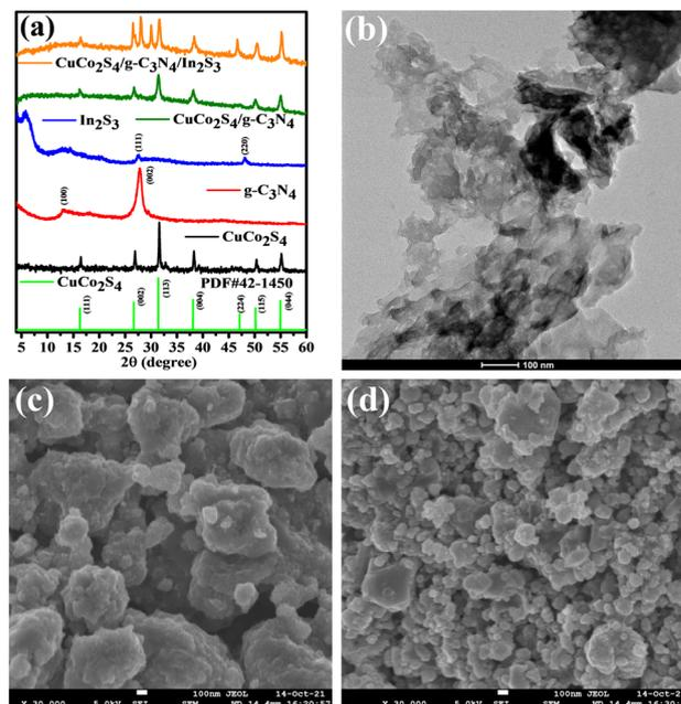
Fig. 1 (a) X-ray diffraction pattern of the as-prepared catalysts; FESEM images (b)  $\text{g-C}_3\text{N}_4$ ; (c)  $\text{CuCo}_2\text{S}_4$ , and (d)  $\text{CuCo}_2\text{S}_4/\text{g-C}_3\text{N}_4/\text{In}_2\text{S}_3$ .
