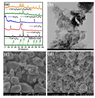
Fig. 1 (a) X-ray diffraction pattern of the as-prepared catalysts; FESEM images (b)  $g-C_3N_4$ ; (c)  $CuCo_2S_4$ , and (d)  $CuCo_2S_4/g-C_3N_4/In_2S_3$ .
