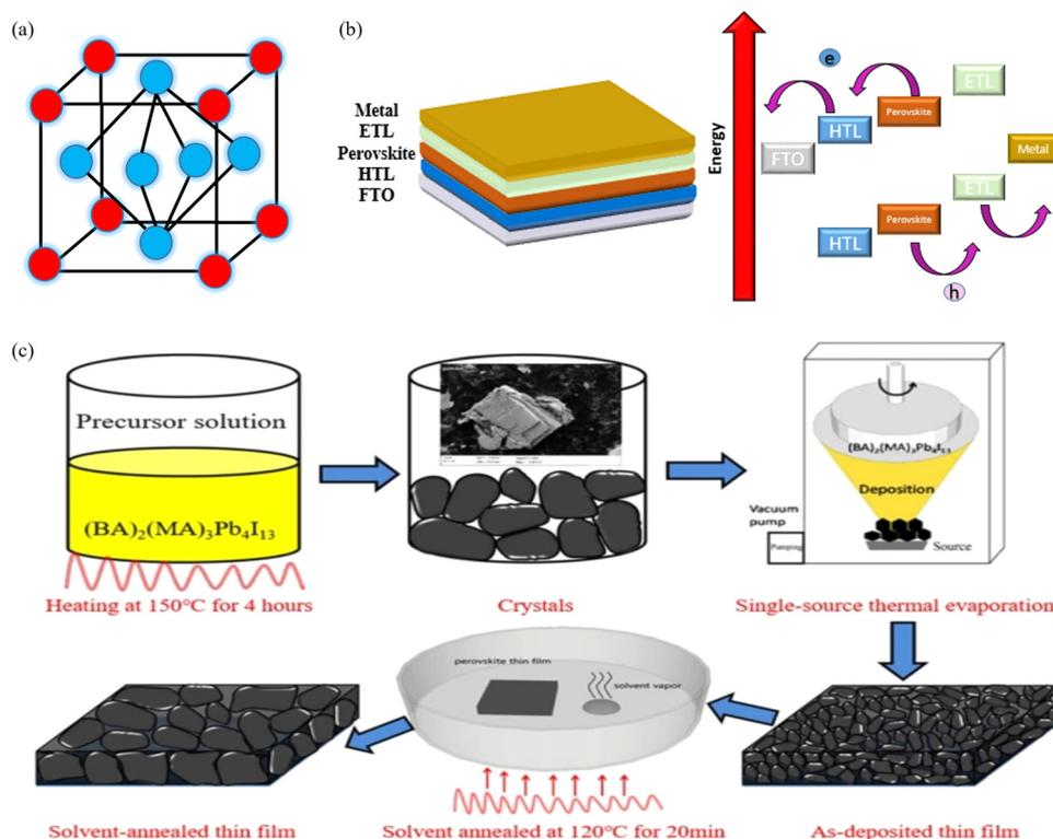
Fig. 8 (a) Unit cell of a perovskite. (b) Working principle of the PSC. (c) Schematic diagram of the fabrication procedure, which includes crystal preparation, single-source thermal evaporation, and solvent annealing (source: Zheng *et al.*,<sup>132</sup> *Sci. Rep.*, Springer Nature, 2019).
