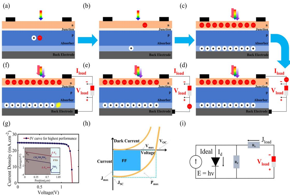
**Fig. 2** (a) Absorption of a single photon of light, (b) generated and separated charge carriers, (c) continuous generation and separation of charge carriers, (d) load is connected, (e) movement of a charge carrier from high potential to low potential, (f) combining electron and holes, (g)  $J$ - $V$  curve, where the inset shows the energy band diagram, (h)  $J$ - $V$  curve, where the inset shows the maximum efficiency, and (i) equivalent electrical model.
