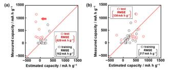
Fig. 2 Relationship between the estimated and measured capacity in the training (black) and test (red) data for models G1 (a) and G2 (b).
