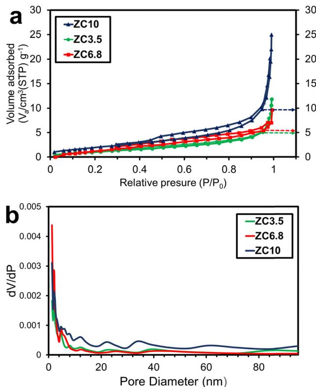
Fig. 5 (a) N<sub>2</sub> adsorption–desorption isotherms and (b) pore size distribution BJH of the samples.
