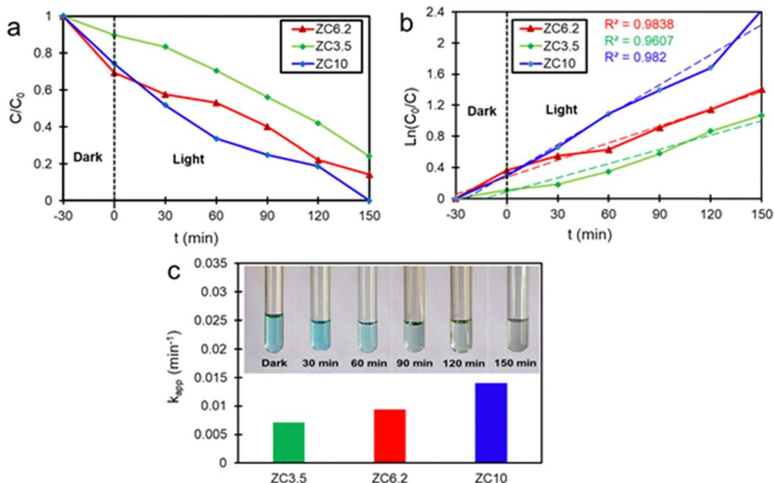
Fig. 7 (a) Photo-degradation rate, (b) plots of  $\ln(C_0/C)$  as a function of visible light time irradiation fitted with a pseudo-first-order kinetic model, and (c) reaction rate constants upon different catalysts exposed to MB.
