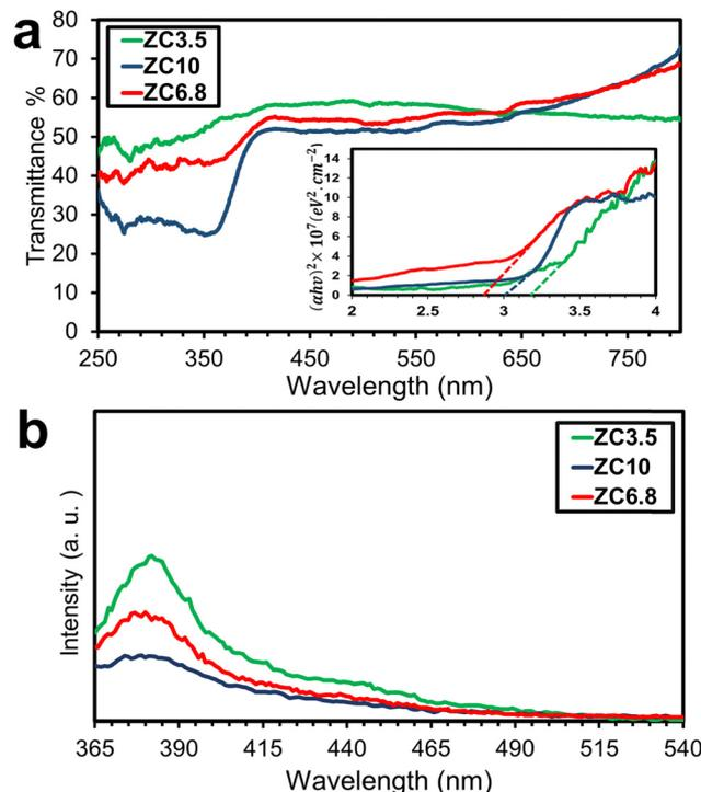
Fig. 6 (a) DRS spectra, Tauc plots for different samples, and (b) room-temperature PL spectra of samples ZC3.5, ZC6.8, and ZC10.
