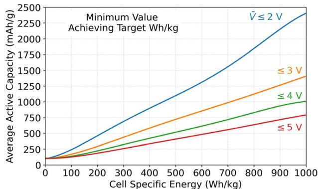
Fig. 4 Minimum average specific capacity (*i.e.*, average of  $Q_{+, \text{act}}$  and  $Q_{-, \text{act}}$ ) capable of achieving specific energy targets (W h kg<sup>-1</sup>), based on results in the Monte Carlo simulation database. Each line represents a different maximum allowable average open circuit voltage ( $\bar{V}$ ).
