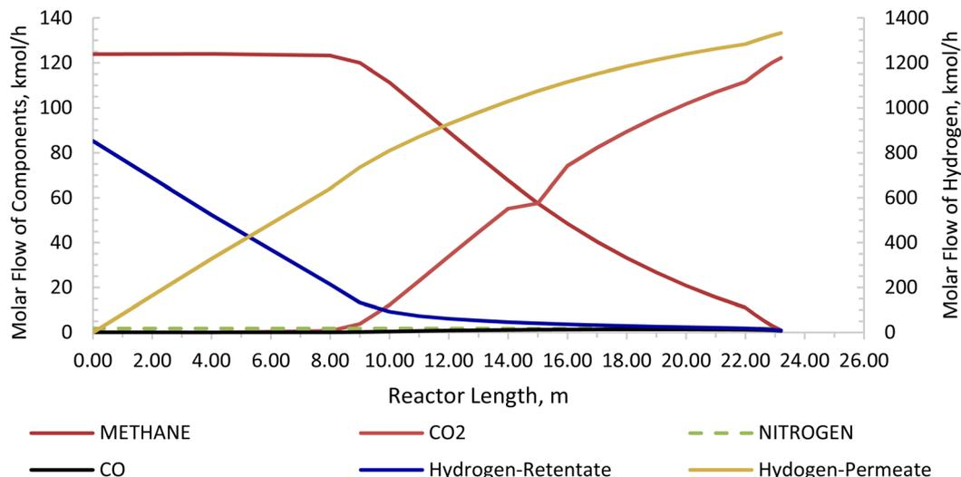
Fig. 12 Membrane reactor product profile for the novel ISEAM process (molar flow of CO<sub>2</sub>, CO, N<sub>2</sub>, H<sub>2</sub>-retentate, and H<sub>2</sub>-permeate).
