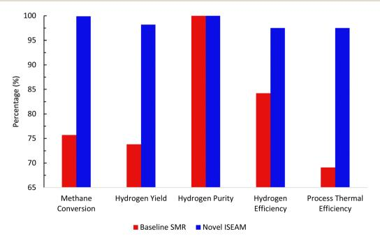
Fig. 10 Comparison between the baseline SMR process and novel ISEAM process
