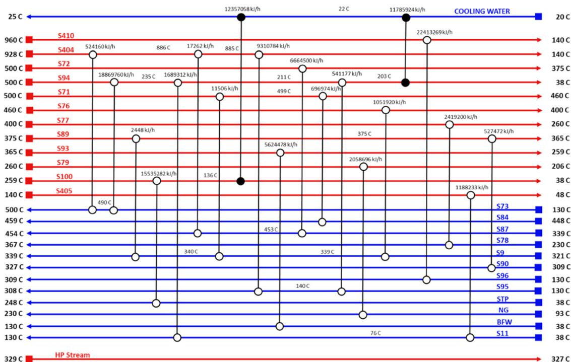
Fig. 6 ISEAM process heat exchanger grid diagram.
