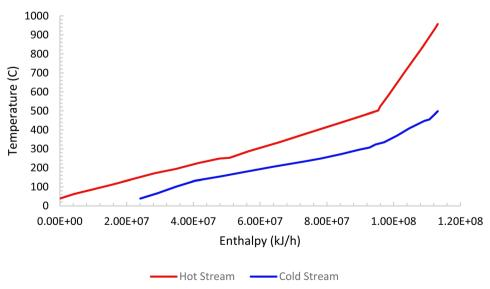
Fig. 5 ISEAM process composite curve.
