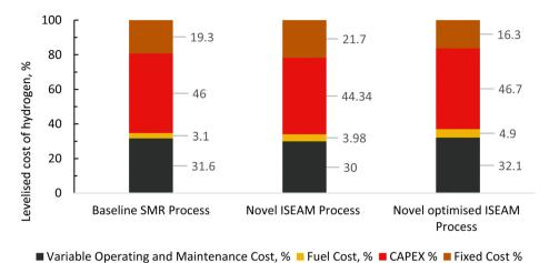
Fig. 16 Distribution of different components of levelized cost (%) for the baseline SMR Process, novel ISEAM and optimised ISEAM process at a fuel cost of \$2.58/MMBTU.
