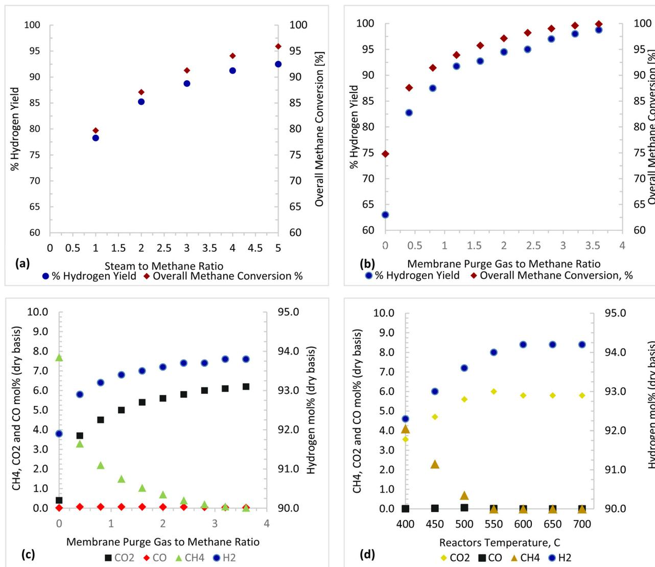
Fig. 13 Parametric investigation results (a) purge gas/ $\text{CH}_4 = 2$ , reactor temperature: 500 °C (b) and (c)  $\text{S}/\text{C} = 3.75$ , reactor temperature: 500 °C, and (d) purge gas/ $\text{CH}_4 = 2$ ,  $\text{S}/\text{C} = 3.75$ .
