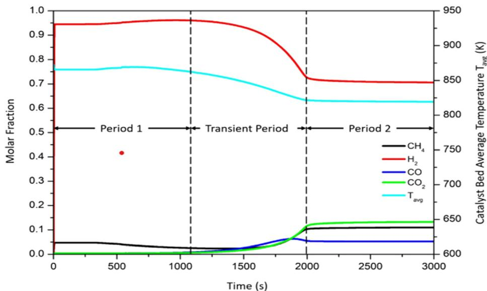
Fig. 4 Typical product plot for 100% sorption enhanced reforming process.<sup>51</sup>
