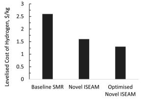
Fig. 14 Levelized cost of hydrogen comparison between baseline SMR process and novel ISEAM process at different fuel cost.
