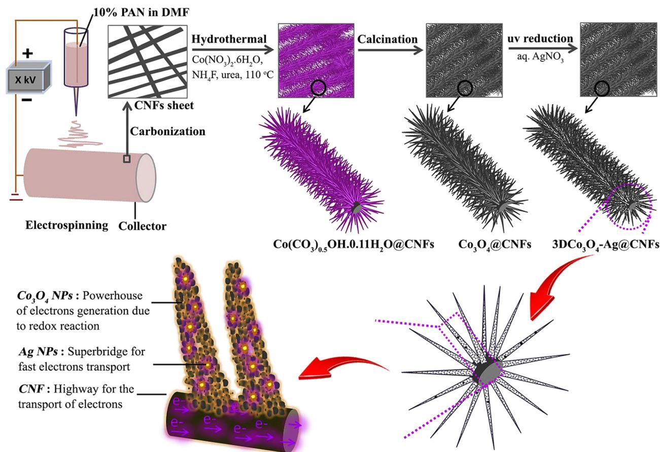
Fig. 15 Schematic representation of 3D  $\text{Co}_3\text{O}_4\text{-Ag}@\text{CNFs}$  nanocomposite electrode preparation, its microstructure and the role of different materials in SC performance. Reproduced from ref. 122 with permission from Elsevier, copyright 2019.
