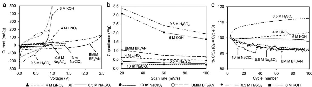
Fig. 5 (a) CV curves for all tested electrolytes ( $100 \text{ mV s}^{-1}$ ). (b) Specific capacitance at different scan rates for each electrolyte. (c) Capacitance retention (% of cycle 3 specific capacitance) over 100 cycles ( $100 \text{ mV s}^{-1}$ ).
