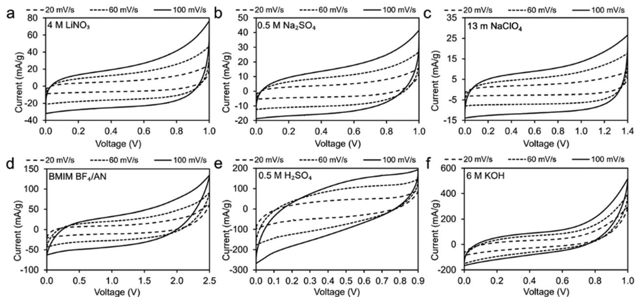
Fig. 4 CV measurements of coal char electrodes in: (a) 4 M  $LiNO_3$ , (b) 0.5 M  $Na_2SO_4$ , (c) 13 m  $NaClO_4$ , (d) BMIM  $BF_4/AN$ , (e) 0.5 M  $H_2SO_4$  and (f) 6 M  $KOH$  at scan rates of 20, 60, and 100  $mV s^{-1}$ .
