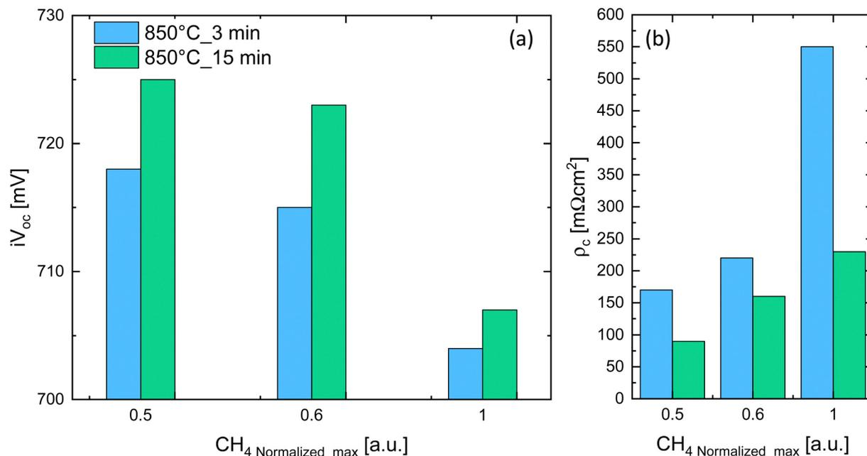
Fig. 1 (a) Implied open circuit voltage ( $iV_{OC}$ ) and (b) specific contact resistance ( $\rho_c$ ) as a function of the CH<sub>4</sub> flow normalized to the maximum value ( $CH_4/CH_{4,max}$ ). The SiC<sub>x</sub>(p) is deposited here on both sides of textured wafers.
