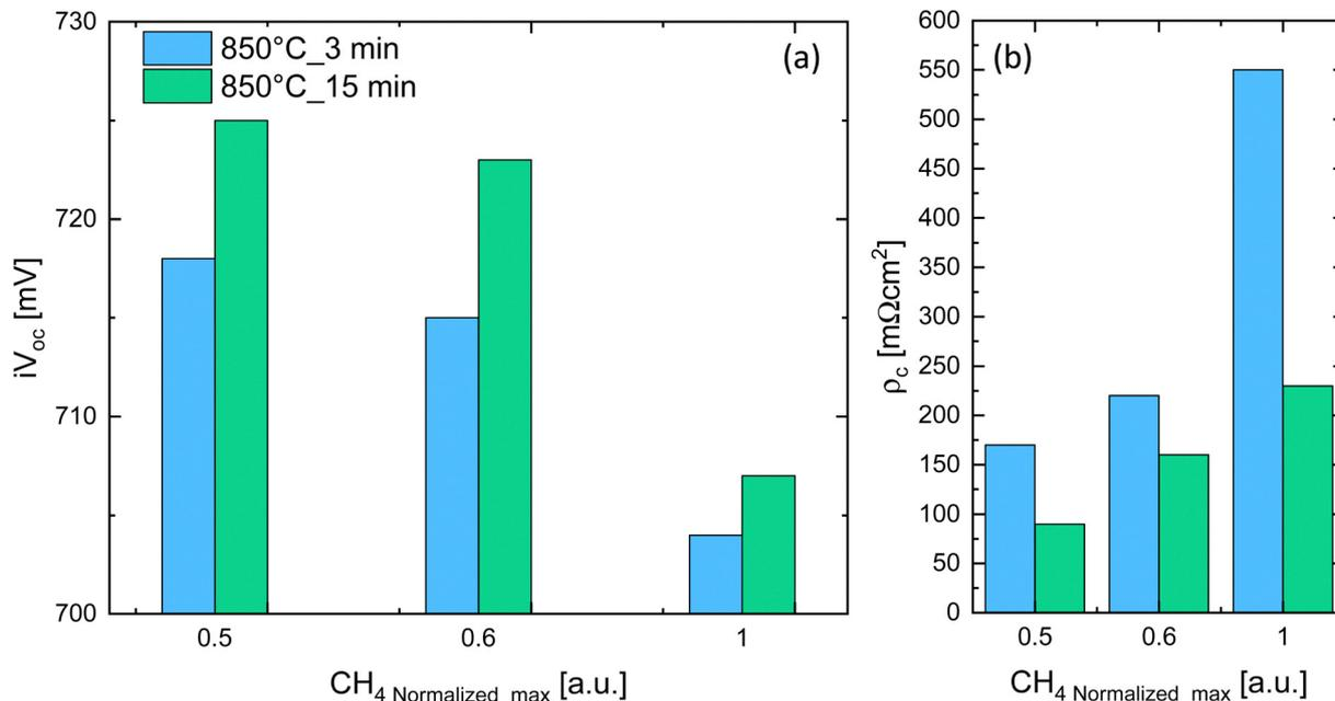
Fig. 1 (a) Implied open circuit voltage ( $iV_{OC}$ ) and (b) specific contact resistance ( $\rho_c$ ) as a function of the  $CH_4$  flow normalized to the maximum value ( $CH_4/CH_{4max}$ ).  $CH_4$  Normalized\_max. The  $SiC_x(p)$  is deposited here on both sides of textured wafers.
