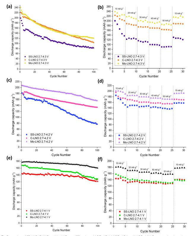
Fig. 7 Comparison of SS-LNO, C-LNO and Mo-LNO over 100 cycles at (a) 2.7–4.3 V, (c) 2.7–4.2 V and (e) 2.7–4.1 V. Rate tests also shown between (b) 2.7–4.3 V, (d) 2.7–4.2 V and (f) 2.7–4.1 V for SS-LNO, C-LNO and Mo-LNO.
