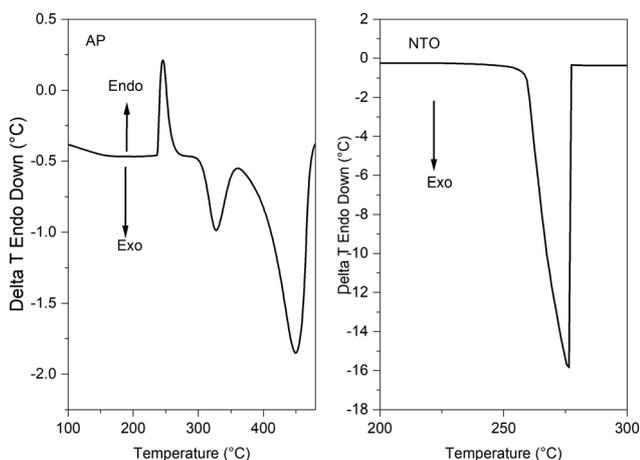
Fig. 7 Thermal decomposition of pure AP and NTO.
