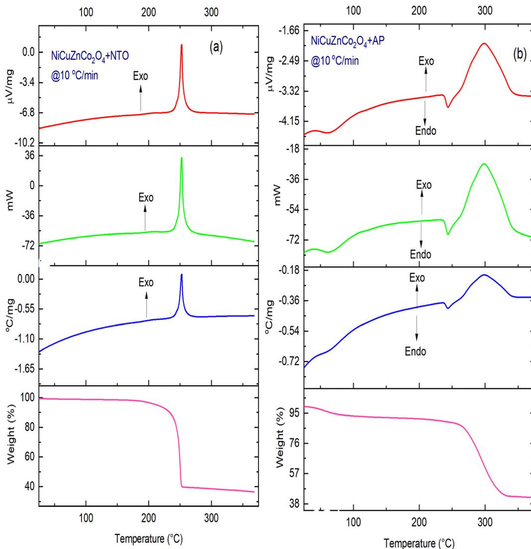
Fig. 8 TG-DTA-DSC thermographs of (a) NiCuZnCo<sub>2</sub>O<sub>4</sub> + NTO and (b) NiCuZnCo<sub>2</sub>O<sub>4</sub> + AP at 10 °C min<sup>-1</sup> heating rate.
