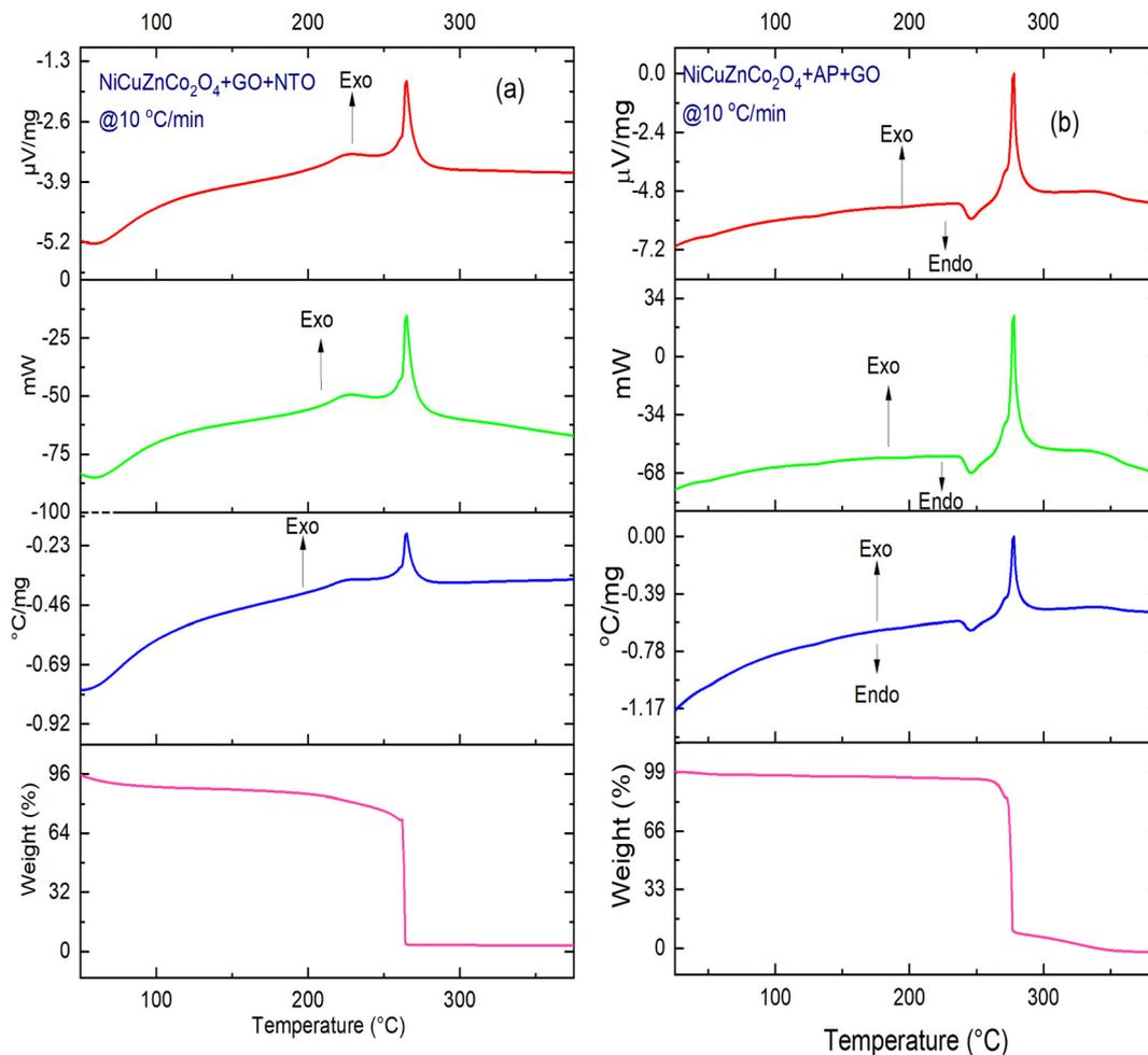
Fig. 9 TG-DTA-DSC thermographs of (a) NiCuZnCo<sub>2</sub>O<sub>4</sub> + GO + NTO and (b) NiCuZnCo<sub>2</sub>O<sub>4</sub> + GO + AP at a heating rate of 10 °C min<sup>-1</sup>.
