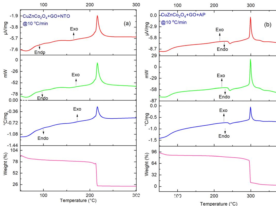
Fig. 11 TG-DTA-DSC thermographs of (a)  $\text{CuZnCo}_2\text{O}_4 + \text{GO} + \text{NTO}$  and (b)  $\text{CuZnCo}_2\text{O}_4 + \text{GO} + \text{AP}$  at a heating rate of  $10\text{ }^\circ\text{C min}^{-1}$ .
