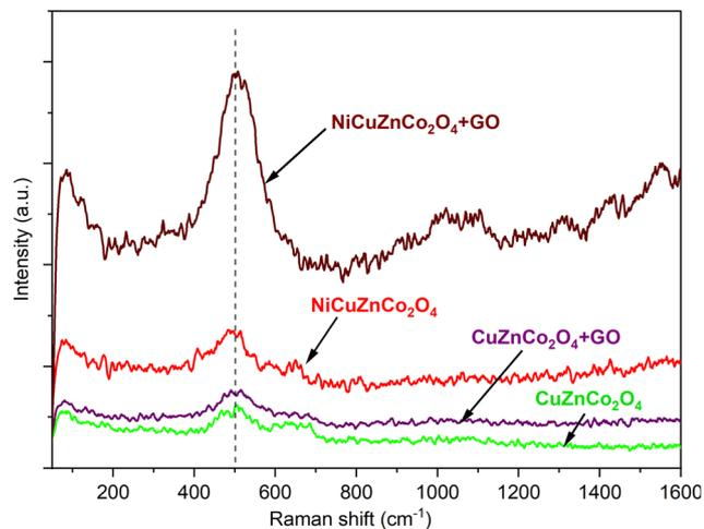
Fig. 4 Raman spectra of NiCuZnCo<sub>2</sub>O<sub>4</sub> + GO, NiCuZnCo<sub>2</sub>O<sub>4</sub>, CuZnCo<sub>2</sub>O<sub>4</sub> + GO, and CuZnCo<sub>2</sub>O<sub>4</sub> cobaltite nanomaterials.
