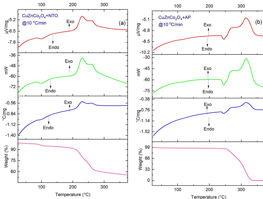
Fig. 10 TG-DTA-DSC thermographs of (a)  $\text{CuZnCo}_2\text{O}_4 + \text{NTO}$  and (b)  $\text{CuZnCo}_2\text{O}_4 + \text{AP}$  at a heating rate of  $10^\circ\text{C min}^{-1}$ .
