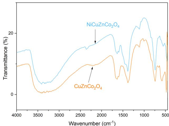
Fig. 5 Fourier transform infrared (FT-IR) spectra of NiCuZnCo<sub>2</sub>O<sub>4</sub> and CuZnCo<sub>2</sub>O<sub>4</sub> cobaltite nanomaterials.
