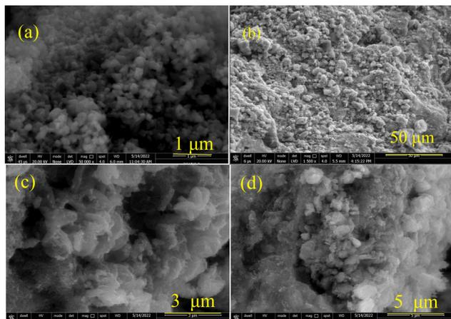
Fig. 6 SEM images of (a) NiCuZnCo<sub>2</sub>O<sub>4</sub>; (b) NiCuZnCo<sub>2</sub>O<sub>4</sub> + GO (c) CuZnCo<sub>2</sub>O<sub>4</sub>; and (d) CuZnCo<sub>2</sub>O<sub>4</sub> + GO.
