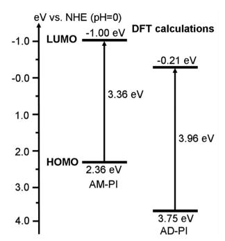
Fig. 6 DFT calculated HOMO and LUMO energy levels of the optimized AM-PI and AD-PI models
