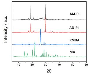
Fig. 2 XRD patterns of AM-PI, AD-PI, PMDA and MA.
