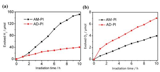
Fig. 8 Time course of (a) H<sub>2</sub> evolution from a 10 vol% aqueous methanol solution by 1 wt% Pt-deposited PI samples and (b) O<sub>2</sub> evolution from a 0.01 M aqueous AgNO<sub>3</sub> solution by bare PI samples. Reaction conditions: 100 mg of PI, visible light irradiation ( $\lambda > 420$  nm)
