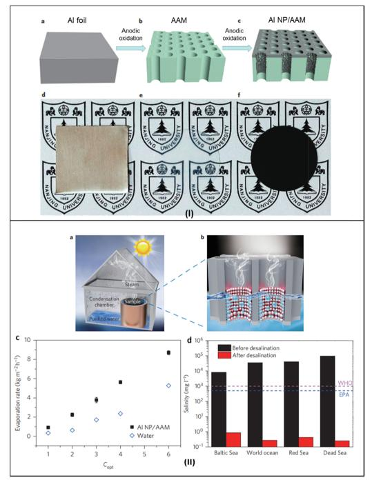
Fig. 7 Plasmonic-based water purification SIWE devices; (I) fabrication process of the Al NP-based plasmonic structure and (II) (a) and b) set-up and schematic of plasmon-enhanced solar desalination, (c and d) performances based on mass change and evaporation rate achieved, respectively, Reproduced with permission.8 Copyright 2016, Springer Nature.
