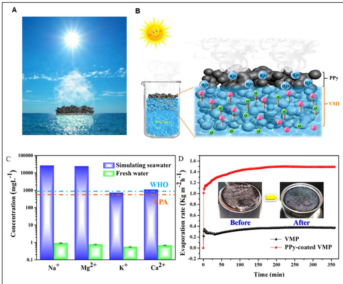
**Fig. 8** Polymer-based water purification SIWE device. (A and B) schematic diagram and structure of the device, (C) concentrations of cations in simulated seawater and distillate; the colored dashed lines denote the WHO and EPA standards for drinkable water, and (D) time-dependent steam evaporation rate in 20 wt% NaCl solution with one sun irradiation. Reproduced with permission.<sup>121</sup> Copyright 2020, American Chemical Society.
