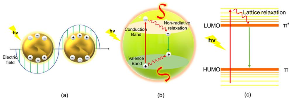
Fig. 3 Different possible photothermal mechanisms: (a) plasmonic heating, (b) electron–hole generation and relaxation, and (c) thermal vibration of molecules.
