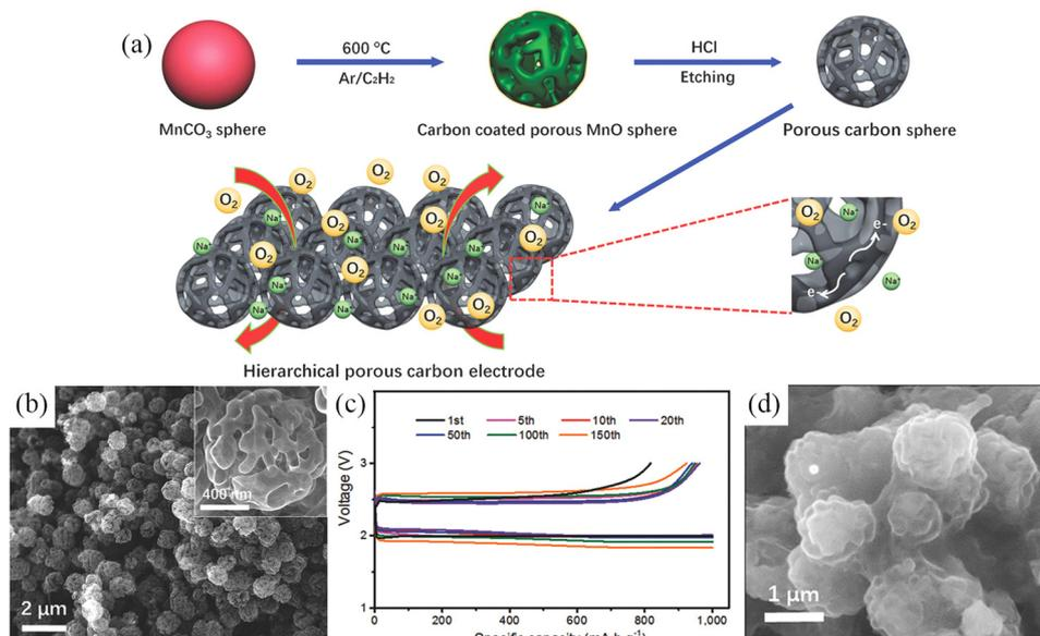
**Fig. 6** (a) Schematic illustration of the synthesis processes of PCS. (b) SEM images of PCS; The inset is a high magnification SEM image of the PCS. (c) Cycling at  $2.0 \text{ A g}^{-1}$  while curtailing the capacity to  $1000 \text{ mA h g}^{-1}$  and (d) SEM image of discharged PCS electrode. (Reproduced from ref. 76 with permission from the WILEY).
