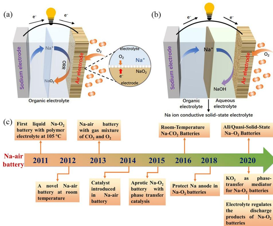
**Fig. 1** Schematic illustration of the operation of: (a) organic Na–air batteries, and (b) hybrid Na–air batteries, (c) the chronology of major events concerning the development of Na–air batteries in the last decade.
