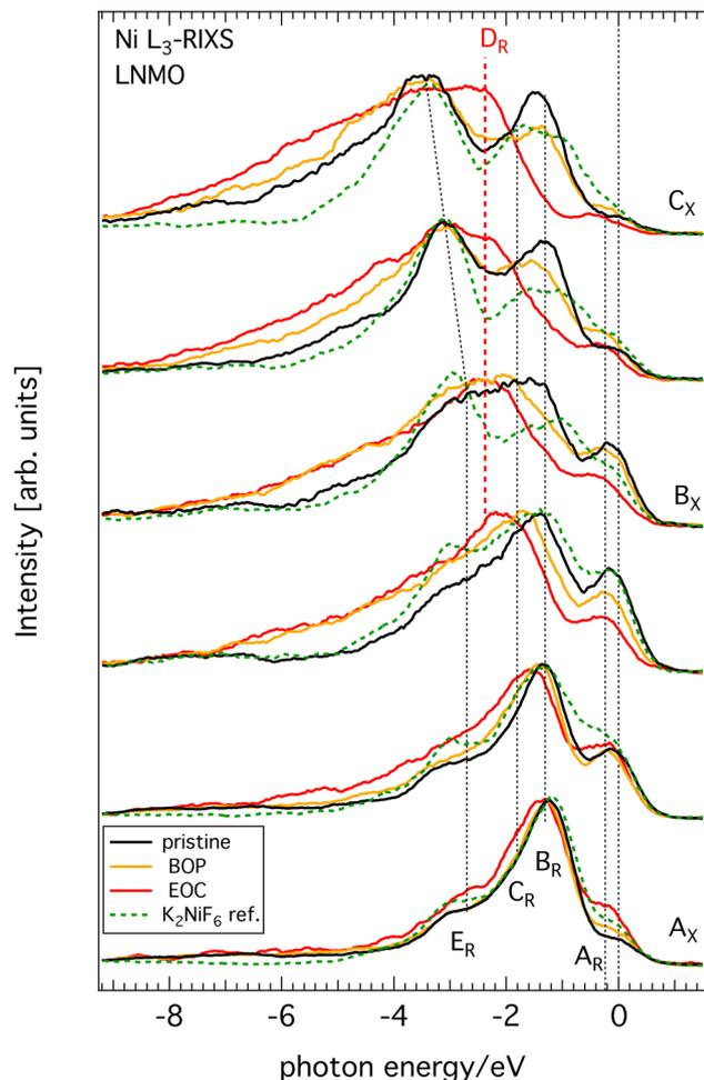
Fig. 5 RIXS spectra across the Ni  $L_3$ -resonances  $A_x$ ,  $B_x$ ,  $C_x$  of  $\text{Li}_{1-x}\text{Ni}_{0.44}\text{Mn}_{1.56}\text{O}_4$  from three selected SoCs and from the Ni(IV) reference compound  $\text{K}_2\text{NiF}_6$  (see color code legend). Each spectrum is normalized to its respective maximum to facilitate spectral shape comparison.
