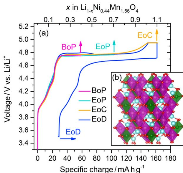
Fig. 1 (a)  $\text{Li}_{1-x}\text{Ni}_{0.44}\text{Mn}_{1.56}\text{O}_4$  charge–discharge profile obtained from the partial curves of the individual cathodes from different states of charge (see text for the definitions): BoP, EoP, EoC, and EoD, respectively. The inset (b) shows the spinel crystal structure in the cation ordered  $P4_332$  space group of  $\text{LiNi}_{0.5}\text{Mn}_{1.5}\text{O}_4$ ; Li (blue), O (red), Ni (green), and Mn (purple).<sup>21</sup>
