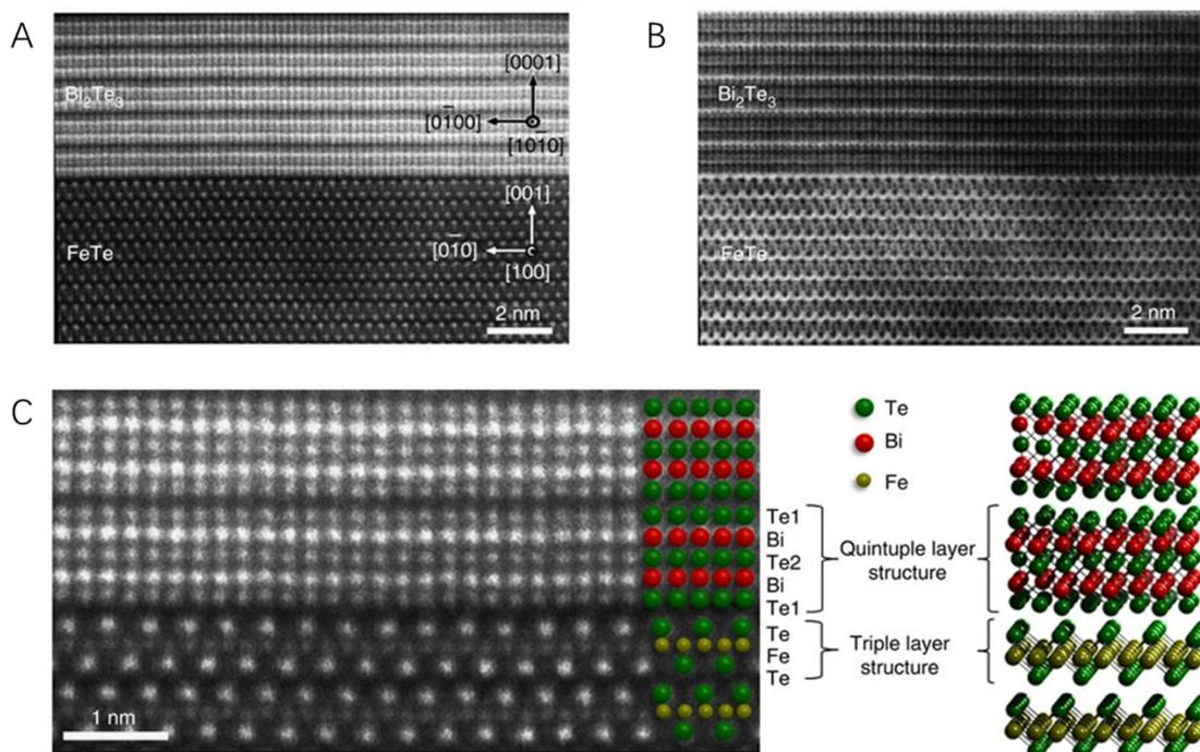
**Fig. 5** The scanning transmission electron microscopy micrographs of a  $\text{Bi}_2\text{Te}_3/\text{FeTe}$  heterostructure. (A) The HADDF image. (B) The annular bright field image. (C) The higher-magnification HADDF image showing the atomically sharp interface between  $\text{Bi}_2\text{Te}_3$  and FeTe. Reproduced with permission from ref. 75, copyright Springer Nature.
