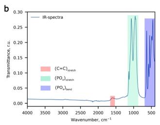
Fig. 1 Spectroscopic measurements. (a) The <sup>57</sup>Fe Mössbauer spectrum, and (b) the FTIR spectrum of Li-rich LFMP
