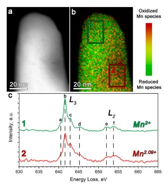
Fig. 2 (a) The ADF-STEM image of  $\text{Li}_{1+\delta}(\text{Fe}_{0.5}\text{Mn}_{0.5})_{1-\delta}\text{PO}_4$  particles with (b) the corresponding color-coded STEM-EELS Mn oxidation state map. (c) The Mn-L<sub>2,3</sub> edge EELS spectra for  $Li_{1+\delta}(Fe_{0.5}Mn_{0.5})_{1-\delta}PO_4$  integrated over the regions 1 and 2, outlined on the image in (b) with green and red rectangles, respectively.
