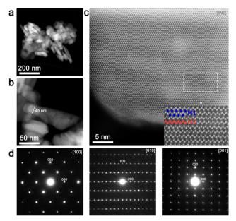
Fig. 3 (a) An overview and (b) the [100] HAADF-STEM image of Li-rich LFMP particles. The minimal thickness along the b-axis (denoted with a double sided arrow) is  $\sim$  45 nm. (c) The low-pass filtered [010] HAADF-STEM image of a Li-rich LFMP crystal; in the magnified area, Fe/Mn atomic columns and Li positions are represented as red and blue circles respectively. (d) The [100], [010] and [001] SAED patterns for Li-rich LFMP.
