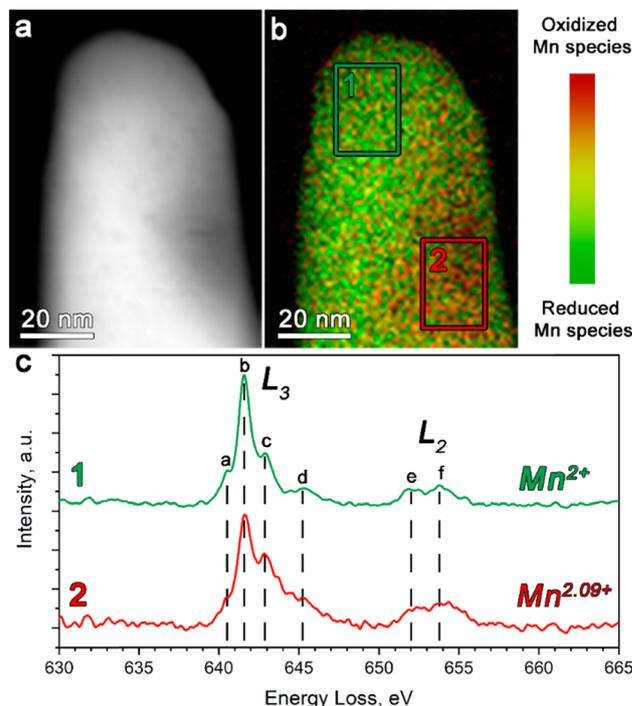
Fig. 2 (a) The ADF-STEM image of  $\text{Li}_{1+\delta}(\text{Fe}_{0.5}\text{Mn}_{0.5})_{1-\delta}\text{PO}_4$  particles with (b) the corresponding color-coded STEM-EELS Mn oxidation state map. (c) The Mn- $L_{2,3}$  edge EELS spectra for  $\text{Li}_{1+\delta}(\text{Fe}_{0.5}\text{Mn}_{0.5})_{1-\delta}\text{PO}_4$  integrated over the regions 1 and 2, outlined on the image in (b) with green and red rectangles, respectively.
