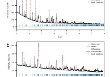
Fig. 4 Crystal structure refinement results. Observed, calculated and difference plots of (a) SXRD and (b) NPD refinement of Li-rich LFMP.
