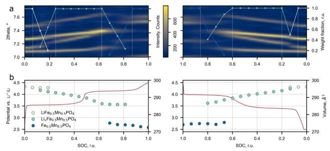
Fig. 6 Synchronized results of operando SXRD study of Li-rich LFMP. (a) Evolution of peak positions and phase weights during cycling. (b) The unit cell volume change during cycling and charge-discharge profile at C/5
