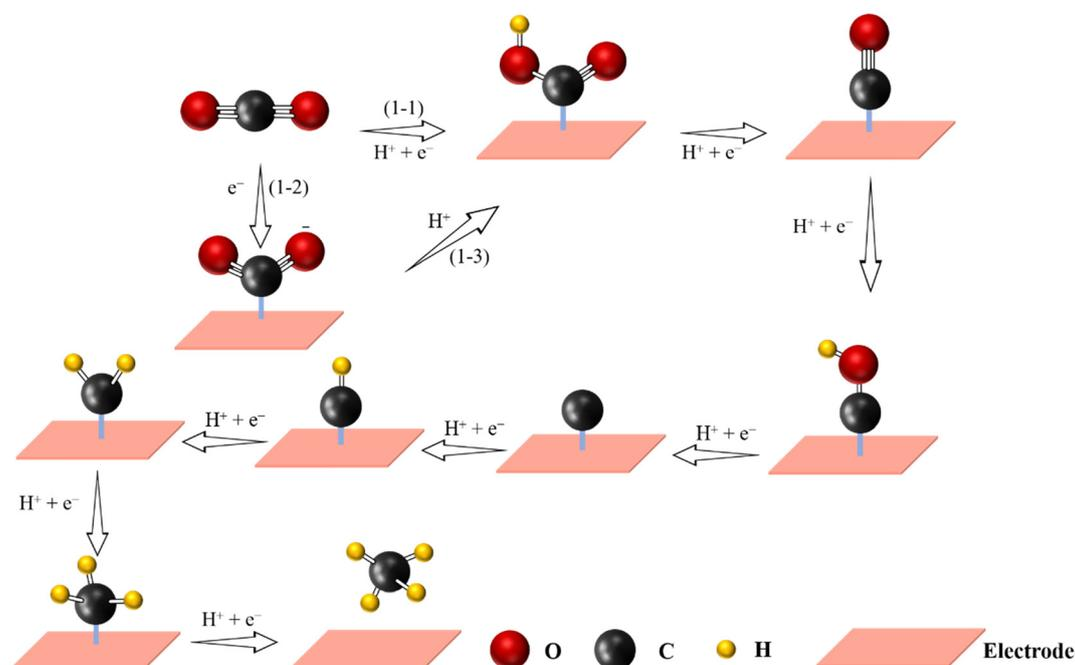
Fig. 7 Proposed reaction pathway for electrochemical CO<sub>2</sub>-to-CH<sub>4</sub> reaction (C atoms: gray; O atoms: red; H atoms: yellow).
