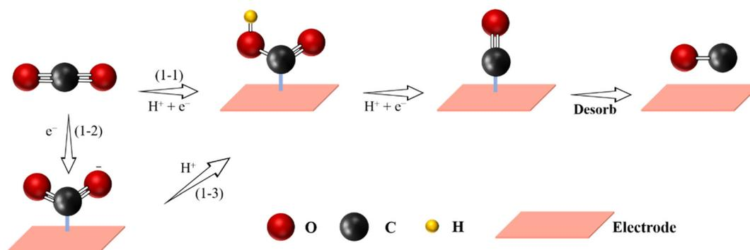
Fig. 4 Proposed reaction pathway for electrochemical CO<sub>2</sub>-to-CO reaction (C atoms: gray; O atoms: red; H atoms: yellow).
