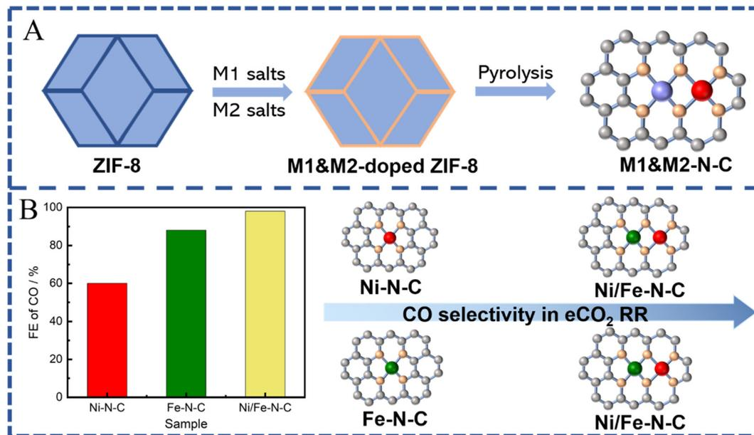
**Fig. 11** (A) Schematic illustration of ZIF-8 derived SACs with two metal sites (C atoms: gray; N atoms: orange; metal atoms: purple/red; heteroatoms: blue). (B) FE of CO (at  $-0.50$  V vs. RHE) obtained on Ni-N-C, Fe-N-C and Ni/Fe-N-C samples (C atoms: gray; N atoms: orange; Ni atoms: red; Fe atom: green).
