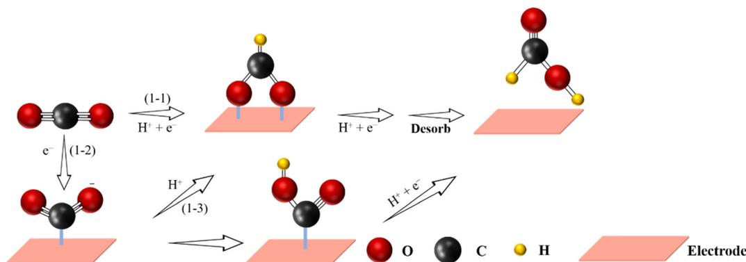
Fig. 5 Proposed reaction pathway for the electrochemical CO<sub>2</sub>-to-HCOOH reaction (C atoms: gray; O atoms: red; H atoms: yellow).
