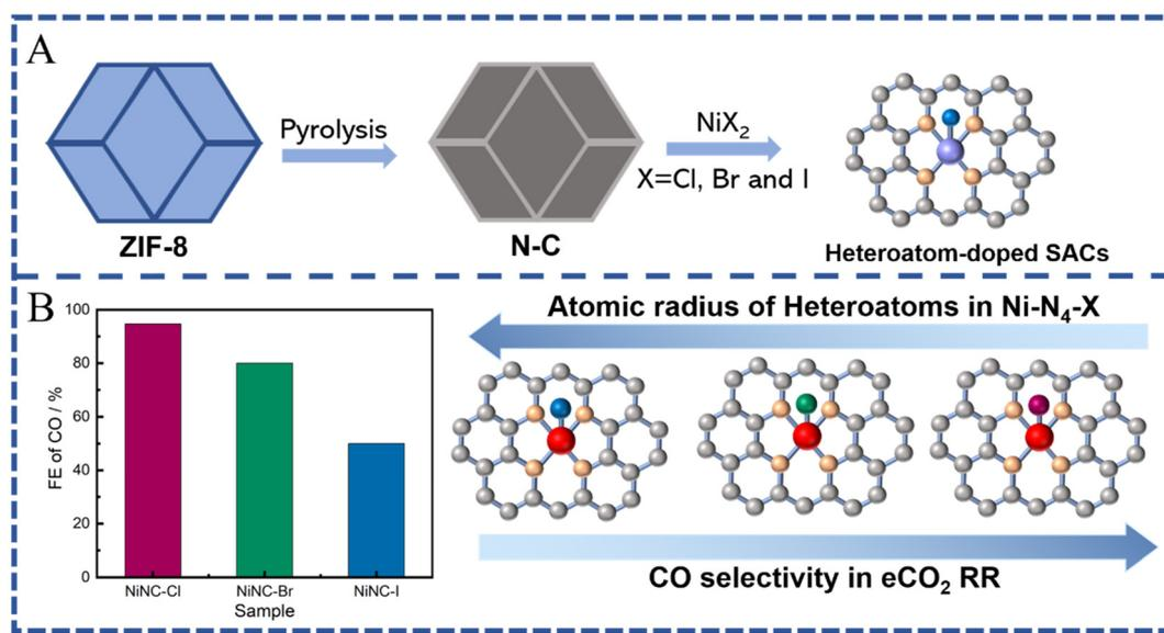
Fig. 10 (A) Schematic illustration of ZIF-8 derived SACs with different heteroatom dopants (C atoms: gray; N atoms: orange; metal atoms: purple/red; heteroatoms: blue). (B) FE of  $\text{CO}$  (at  $-0.7$  V vs. RHE) obtained on Ni-SACs with different heteroatom dopants (C atoms: gray; N atoms: orange; Ni atoms: red; Cl atom: dark red; Br atom: green; I atom: dark blue).
