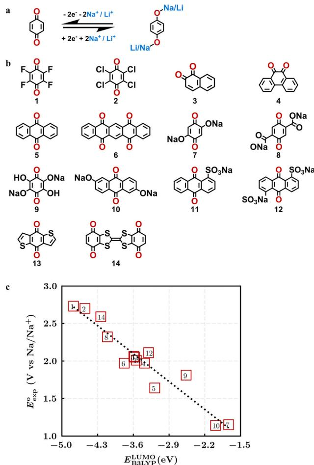
**Fig. 2** (a) A representation of the quinone reaction with metal ions at the cathodes of sodium- and lithium-ion batteries; (b) 2D structural representations of the fourteen experimentally studied quinones that have been used to develop an equation of calibration between the physicochemical descriptors and the reduction potentials; (c) observed performance of the DFT-optimized reactant molecule LUMO-energy as a descriptor for the prediction of measured reduction potentials in experiments.
