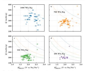
Fig. 4 The distribution of the gravimetric charge capacity versus reduction potential for: (a) one-ring, (b) two-ring, (c) three-ring, and (d) four-ring compounds. Only the calculation data for 289 likely stable quinones, which have  $RMSD_C \leq t_b$ , are shown. The dotted blue, orange, green, and purple lines represent the cut-off energy density values for the group of molecules with increasing number of rings, respectively, from one to four
