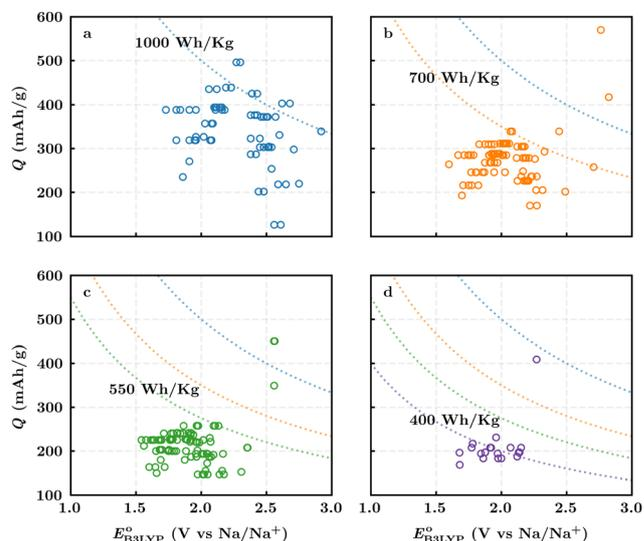
Fig. 4 The distribution of the gravimetric charge capacity *versus* reduction potential for: (a) one-ring, (b) two-ring, (c) three-ring, and (d) four-ring compounds. Only the calculation data for 289 likely stable quinones, which have  $\text{RMSD}_{\text{C}} \leq t_{\text{b}}$ , are shown. The dotted blue, orange, green, and purple lines represent the cut-off energy density values for the group of molecules with increasing number of rings, respectively, from one to four.
