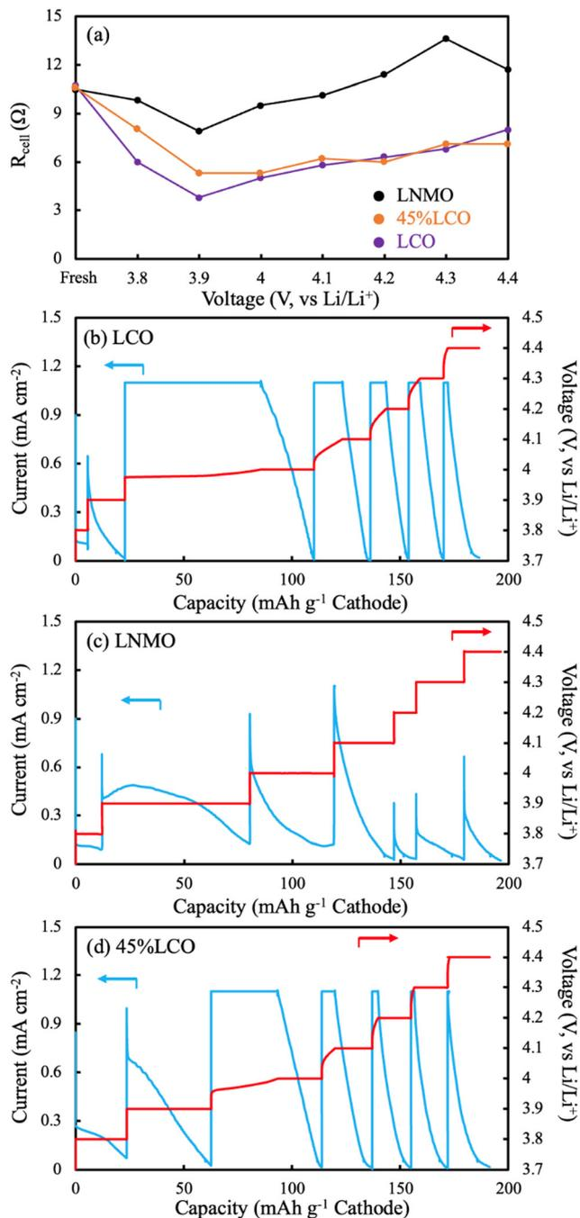
Fig. 7 (a)  $R_{\text{cell}}$  as a function of voltage for AAM LNMO (black), AAM 45%LCO (orange), and AAM LCO (purple). Values were obtained by fitting EIS Nyquist plots. EIS was conducted after the voltage hold step of a CCCV charge of a cell with the indicated cathode paired with a lithium metal anode. The CCCV charge outcomes are displayed for the relevant cells with (b) LCO, (c) LNMO, and (d) 45%LCO, where red and blue curves represent the voltage and the current density, respectively.
