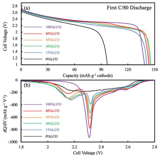
**Fig. 3** (a) Discharge voltage profiles at low rate for AAM electrode cells containing LTO anodes and cathodes comprised of 100%LCO (purple), 60%LCO (red), 45%LCO (orange), 30%LCO (green), 15%LCO (blue), and 0%LCO (black). The discharge was at a rate of C/80, which was the same rate used for the charge cycle and corresponded to  $\sim 0.282 \text{ mA cm}^{-2}$ . (b) The corresponding dQ/dV plots calculated from the discharge results shown in (a).
