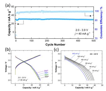
Fig. 4 Electrochemical properties of  $K_{0.6}Cr_{0.6}Ti_{0.4}O_2$  as a potential positive electrode material for KIBs; (a) cycling stability for 500 cycles in the potential range of 2.0-3.9 V, (b) corresponding charge/discharge curves at the 200th, 300th, 400th, and 500th cycles, and (c) rate capability (active material mass loading:  $2.16 \text{ mg cm}^{-2}$ ).
