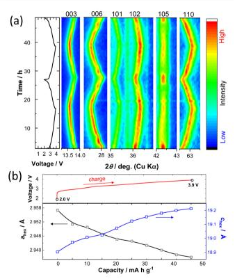
Fig. 3 Structural changes of  $K_{0.6-y}Cr_{0.6}Ti_{0.4}O_2$  during charge/discharge; (a) the contour plots of in situ XRD data during the first two cycles in the voltage range of 2.0-3.9 V at a rate of 4 mA  $g^{-1}$ . The voltage change of the in situ cell is also shown. (b) Lattice parameter variations during the 2nd
