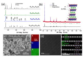
Fig. 1 Structural characterization of  $K_xCr_xTi_{1-x}O_2$ ; (a) the XRD patterns of  $K_xCr_xTi_{1-x}O_2$  with different chemical compositions, (b) the Rietveld refined XRD pattern of  $K_{0.6}Cr_{0.6}Ti_{0.4}O_2$  and a schematic illustration of the P3-type layered structure is also shown in the inset, (c) the FE-SEM image and EDX maps of  $K_{0.6}Cr_{0.6}Ti_{0.4}O_2$ , and (d) the HAADF-STEM images of  $K_{0.5}Cr_{0.5}Ti_{0.5}O_2$
