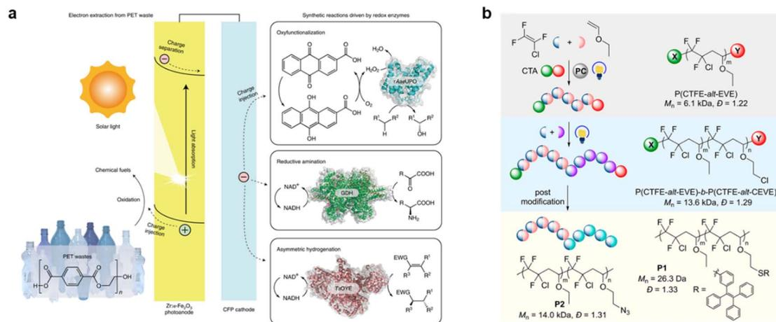
Fig. 7 (a) CFP-based cathodes reduce  $O_2$  to  $H_2O_2$  for biocatalytic oxyfunctionalization and  $NAD^+$  to  $NADH$  for enzymatic amination and asymmetric hydrogenation. Reproduced with permission from ref. 152 Copyright 2022, Springer Nature. (b) Synthetic schemes of the two-step photopolymerization and post-modification. Reproduced with permission from ref. 155 Copyright 2020, ACS.
