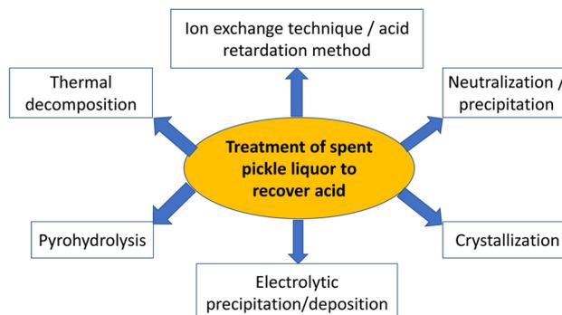
Fig. 3 Different techniques and methodologies employed for the regeneration and recovery of acids from the spent pickle liquors.
