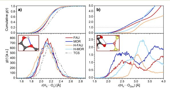
Fig. 4 Radial distribution functions (RDFs) obtained from AIMD simulations. (a) Intramolecular hydrogen bonds of TCS, (b)  $H_h \cdots O_{Zeo}$  hydrogen bonds. Top panels show the cumulative RDFs.
