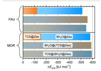
Fig. 7 Boltzmann-averaged adsorption energies obtained for all-silica FAU and MOR with co-adsorbed TCS and water. Sums of the adsorption energies of individual guest molecules are shown for comparison (top columns).
