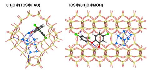
Fig. 8 Lowest-energy configurations of co-adsorbed TCS and water in all-silica zeolites FAU and MOR. Oxygen atoms of H<sub>2</sub>O molecules are shown in blue.
