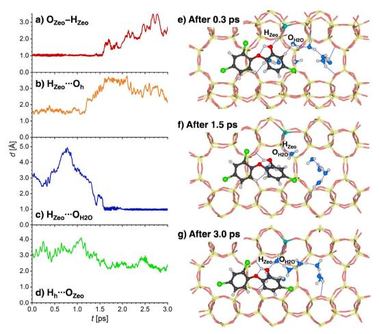
Fig. 9 (a)–(d) Evolution of selected interatomic distances during the first 3 ps of one AIMD trajectory (Traj1) computed for 8H<sub>2</sub>O@(TCS@H-MOR), (e)-(g) environment of the framework Al atom at different stages of the simulation.
