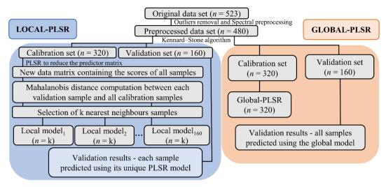
Fig. 3 Flow chart of LOCAL-PLSR and GLOBAL-PLSR calibration procedures. For a given sample in the validation set, k is the number of nearest neighbor samples selected in the calibration set considering a given Mahalanobis limit distance.
