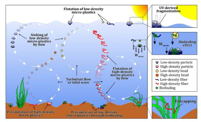
Schematic of MP settling behavior affected by different parameters
