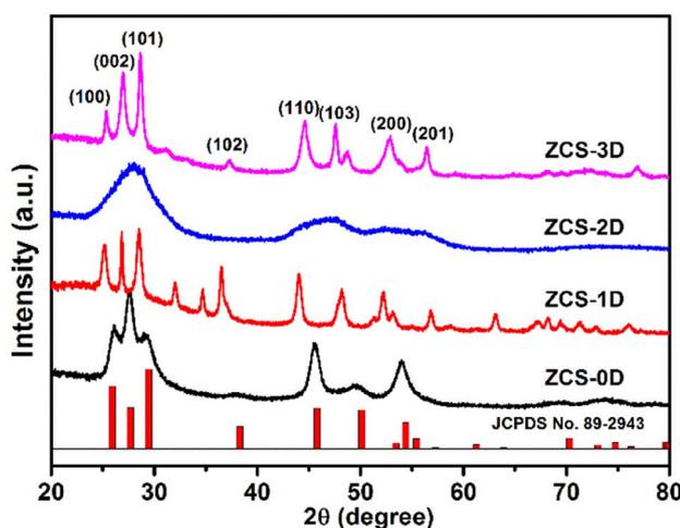
Fig. 1 XRD patterns of synthesized Zn<sub>0.5</sub>Cd<sub>0.5</sub>S nanomaterials with different morphologies.
