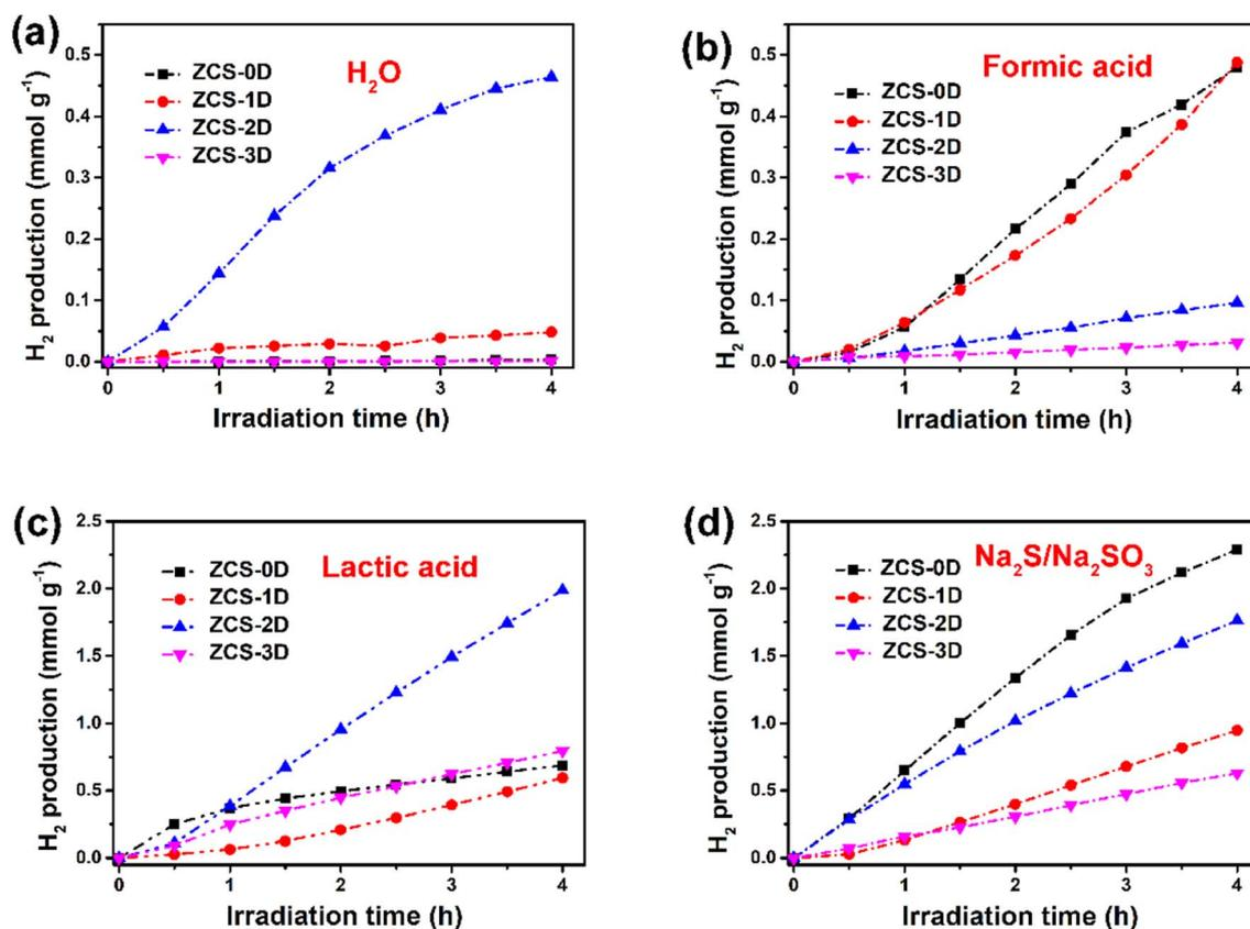
Fig. 5 Photocatalytic  $\text{H}_2$  production of ZCS samples in different solvents:  $\text{H}_2\text{O}$  (a), formic acid (b), lactic acid (c), and  $\text{Na}_2\text{S}/\text{Na}_2\text{SO}_3$  (d).
