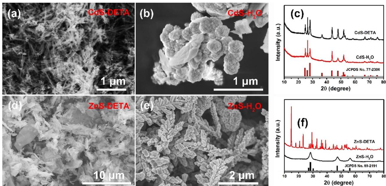
Fig. 4 SEM images of CdS-DETA (a), CdS-H<sub>2</sub>O (b), ZnS-DETA (d), and ZnS-H<sub>2</sub>O (e), and XRD patterns of CdS (c) and ZnS (f) with different solvent syntheses.
