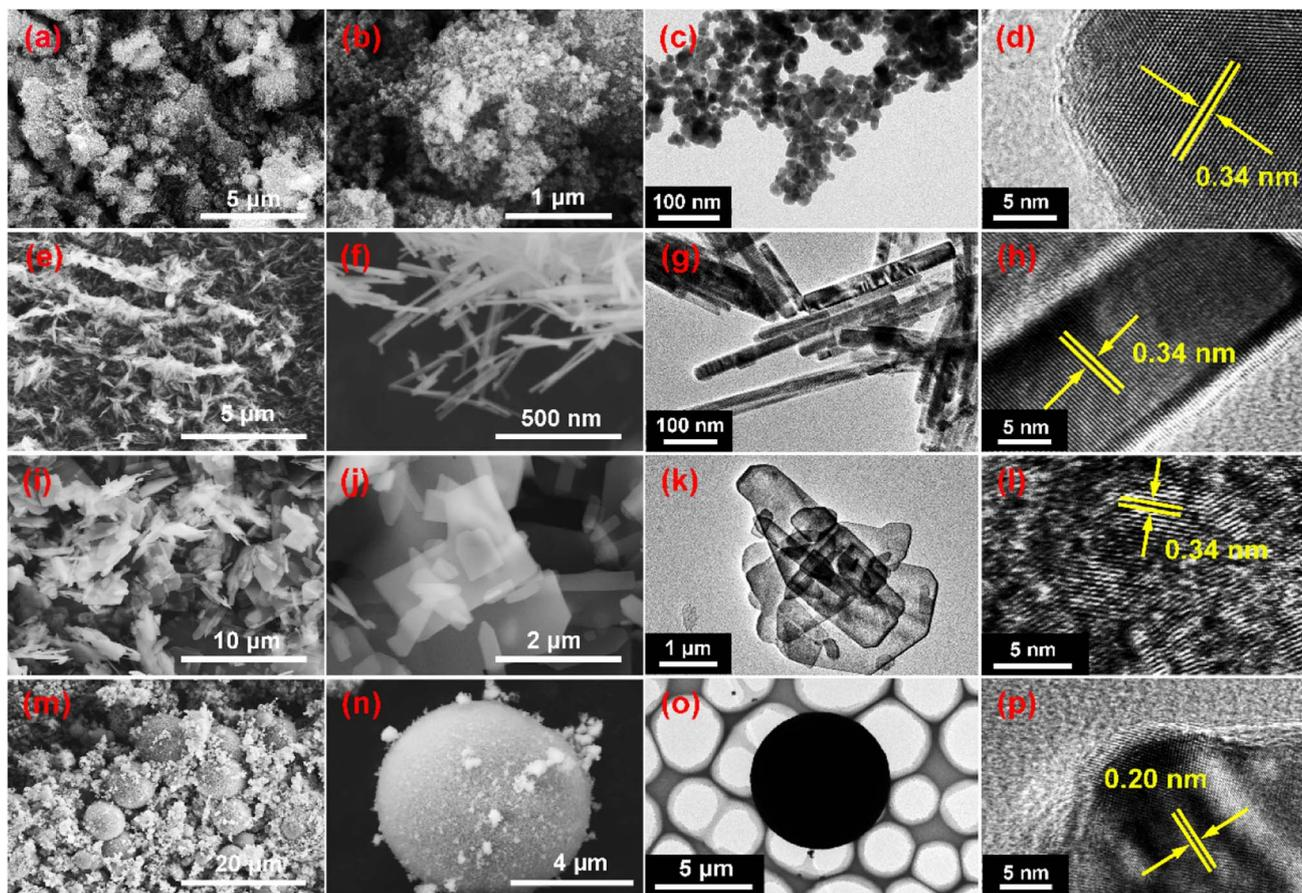
Fig. 2 SEM images of the synthesized  $\text{Zn}_{0.5}\text{Cd}_{0.5}\text{S}$  nanomaterials with different shapes: ZCS-0D (a–d), ZCS-1D (e–h), ZCS-2D (i–l), and ZCS-3D (m–p).
