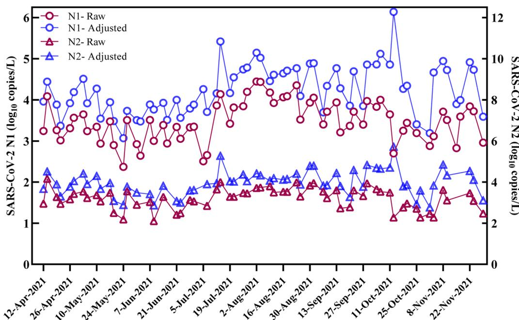
Fig. 2 Concentrations of SARS-CoV-2 N1 and N2 ( $\log_{10}$  copies per L) in raw and BCoV recovery adjusted influent samples.
