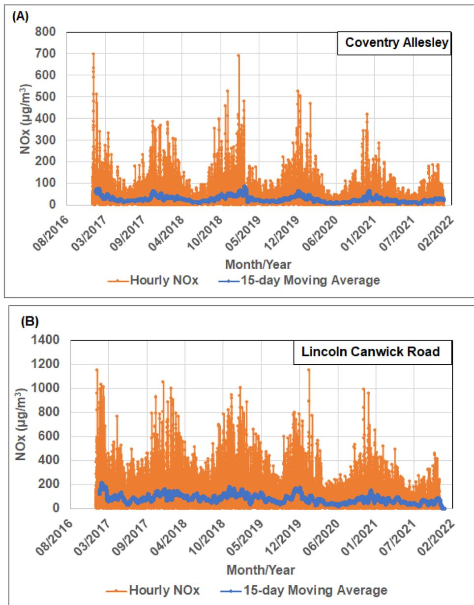
Fig. 2 Hourly NO<sub>x</sub> recorded data at two city sites from Central England from 2017 to 2021: (A) Coventry Allesley (typical of urban background recordings); (B) Lincoln Canwick Road (typical of urban roadside recordings). The trends displayed highlight that both types of recording site display multiple short-lived NO<sub>x</sub> peaks (spikes) with higher background and peak values occurring at the roadside site.
