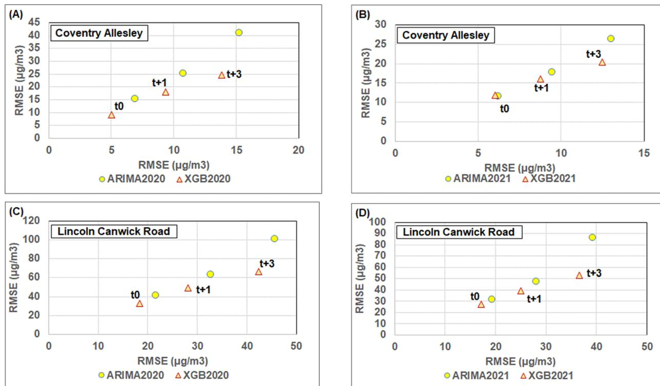
Fig. 10 ARIMA and XGB NO<sub>x</sub> air quality prediction errors compared for time periods  $t_0$ ,  $t + 1$  and  $t + 3$  for the Coventry Allesley site: (A) 2020; and, (B) 2021; and the Lincoln Canwick Road site: (C) 2020; and, (D) 2021. The XGB trend-attribute models outperform ARIMA models for the urban background and roadside sites evaluated.
