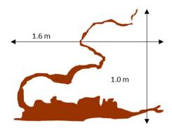
Fig. 4 Left, view of the precipitated iron barrier through the Perspex® plastic sides of the large scale experiment; right, superimposable schematic of the iron barrier with approximate dimensions.
