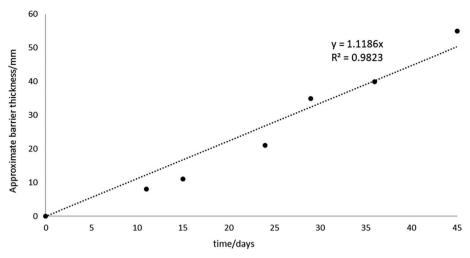
Fig. 10 Barrier growth over time, showing a strong correlation ( $R^2 = 0.98$ ) between barrier thickness and time over which voltage is applied to the system (1.25 kg sand, LWH =  $19 \times 13 \times 9$  cm cells, 500 ppm KCl electrolyte at 10 V, or 0.53 V cm<sup>-1</sup>).
