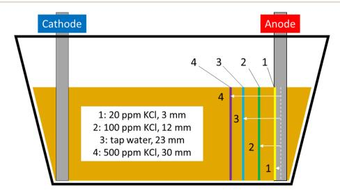
Fig. 9 Scaled schematic of the EKR test cells with lines showing distance from anode at which iron barrier material was first observed; 1 = 20 ppm KCl electrolyte, 2 = 100 ppm KCl electrolyte, 3 = 100 ppm KCl electrolyte.
