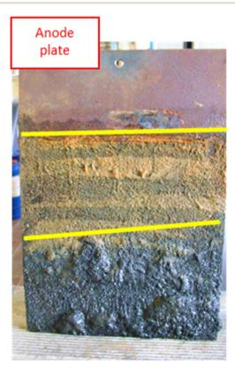
Fig. 6 Cathode (left) and anode (right) plates from a pilot scale experiment (described in ESI $\dagger$ ), conducted to inform set-up of the large-scale experiment, showing the difference in galvanic corrosion. The distinct bands of material are highlighted on the anode with yellow lines. Dimensions: LWH 0.2  $\times$  28  $\times$  18 cm.
