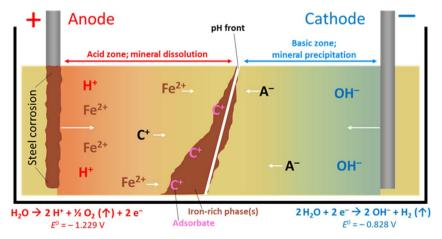
Fig. 1 The FIRS process, with precipitation of iron-rich phases. Cation (C<sup>+</sup>) and anion (A<sup>-</sup>) movement with pH gradient, towards electrodes of opposing charge, is shown. Water electrolysis half-cell values are vs. SHE. The oxidation of ferrous to ferric iron (Fe<sup>2+</sup> to Fe<sup>3+</sup>  $E^{\circ} = -0.771 \text{ V}$  vs. SHE)<sup>24</sup> typically occurs by diffusion of dioxygen through interstitial pore waters. System uses direct current application.
