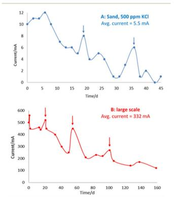
Fig. 7 A (top) and B (bottom) - Amperometry for cell with 500 ppm KCl in sand (top, "A") and large-scale experiment (bottom, "B"). Vertical arrows indicate addition of electrolyte and corresponding current increase. Avg. is average
