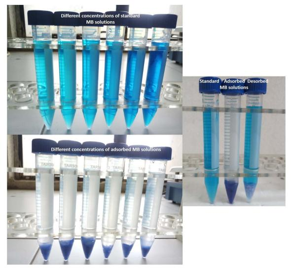
Pictorial representation of adsorbed and desorbed methylene blue samples along with standard solutions of the dye.
