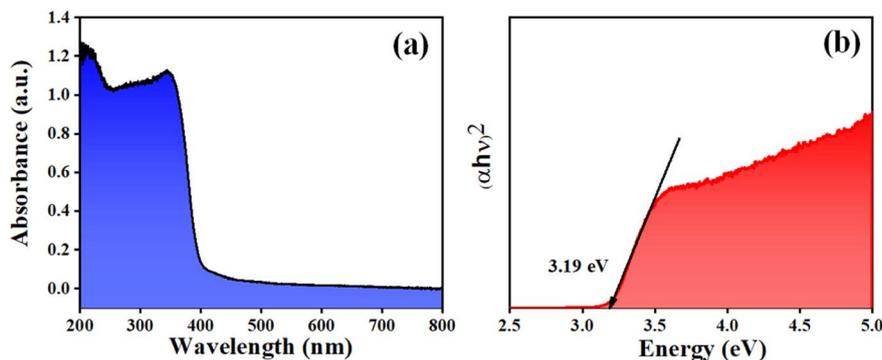
Fig. 3 (a) DRS of BaTiO<sub>3</sub>, (b) Tauc's plot for energy band gap.
