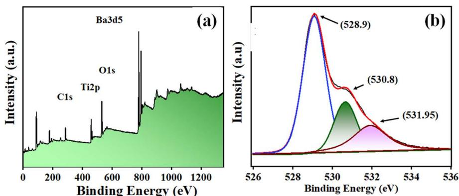
Fig. 4 (a) XPS survey of BaTiO<sub>3</sub>, (b) deconvoluted survey of O 1s.
