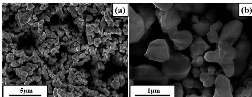
Fig. 2 SEM images of synthesized BaTiO<sub>3</sub> at a resolution scale of (a) 5 μm, (b) 1 μm.
