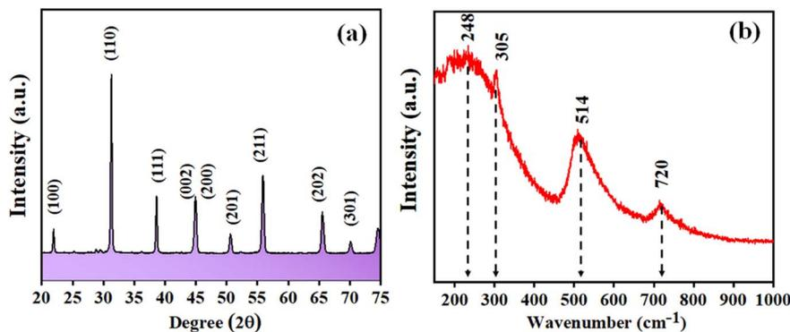
Fig. 1 Synthesized BaTiO<sub>3</sub> (a) XRD pattern, (b) Raman spectrum.
