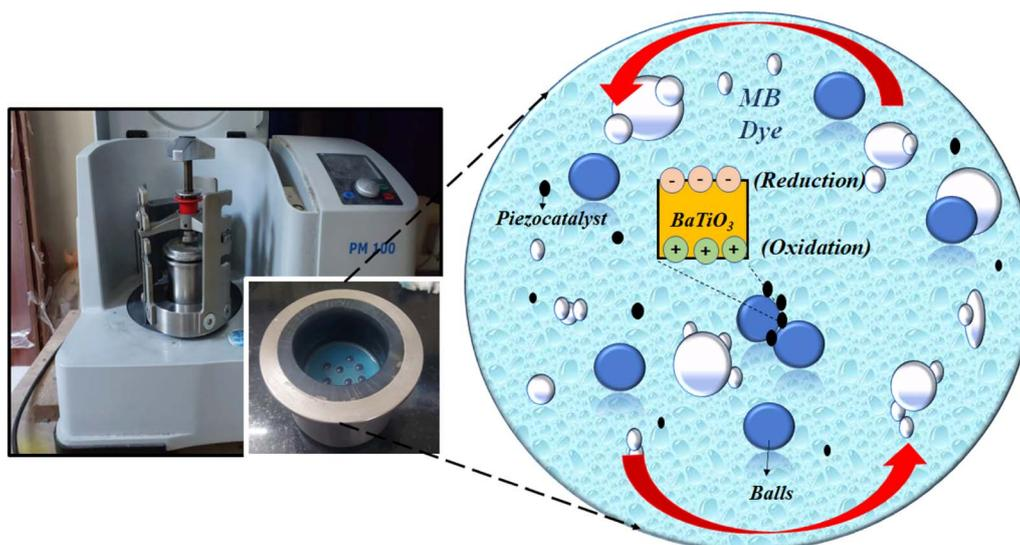
Fig. 9 Schematic representation of piezocatalysis process induced from ball milling for MB dye degradation.
