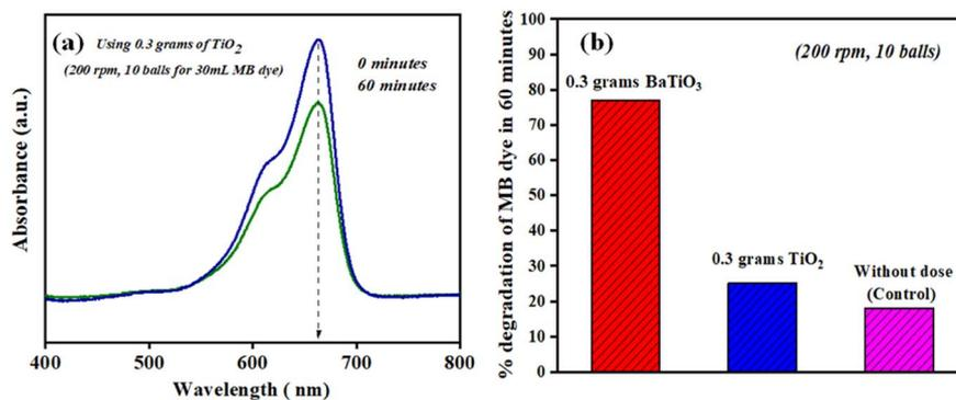
Fig. 8 (a) Absorbance spectra of MB dye using 0.3 g of  $\text{TiO}_2$  (non-piezoelectric material) in 60 min with ball milling at 200 rpm using 10 balls, (b) % degradation of MB dye in 60 min using 0.3 g of  $\text{BaTiO}_3$ ,  $\text{TiO}_2$ , and without using any catalyst in 60 min with ball milling at 200 rpm using 10 balls.
