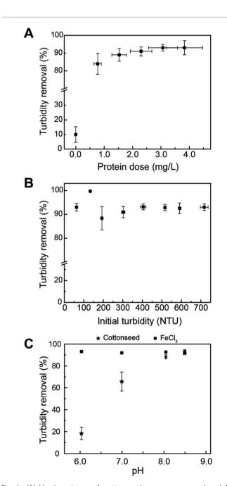
Fig. 1 (A) Varying doses of cottonseed serum were analyzed for turbidity removal. (B) Initial turbidity ranging from 62.5-717 NTU was investigated for the effect on coagulation. (C) Various pH values were analyzed for turbidity removal using cottonseed serum and FeCl3.
