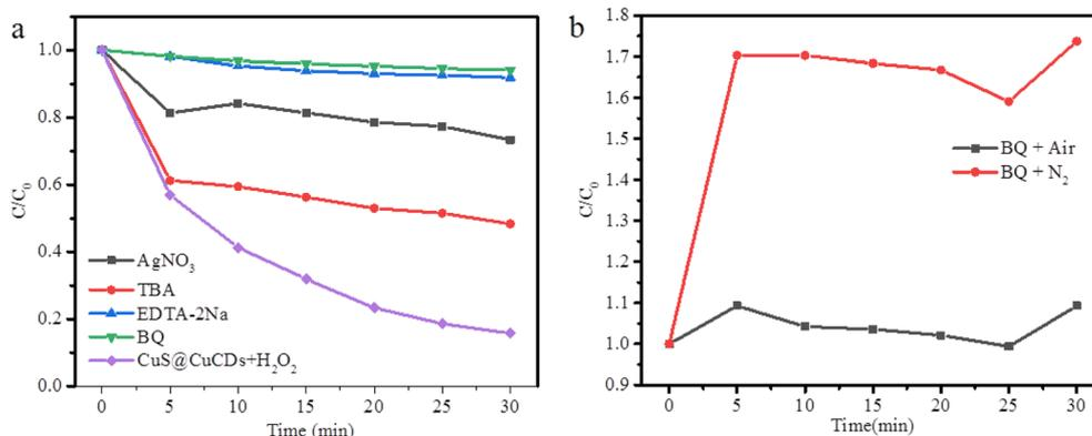
Fig. 8 (a) Active species trapping experiments and (b)  $\cdot\text{O}_2^-$  quenching experiments under air and the solution treated with N<sub>2</sub> before the reaction on TC Fenton-like photodegradation by CuS@Cu-CDs [catalyst dosage] = 20 mg; [H<sub>2</sub>O<sub>2</sub>] = 7 mM; [TC] = 20 mg L<sup>-1</sup>; pH = 5.6.
