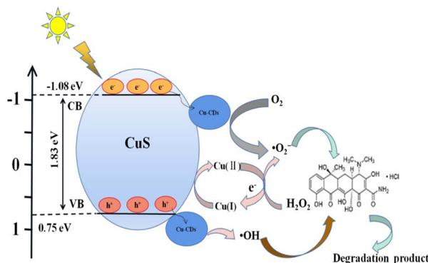
Scheme 2 Proposed mechanism of photocatalytic degradation of TC.
