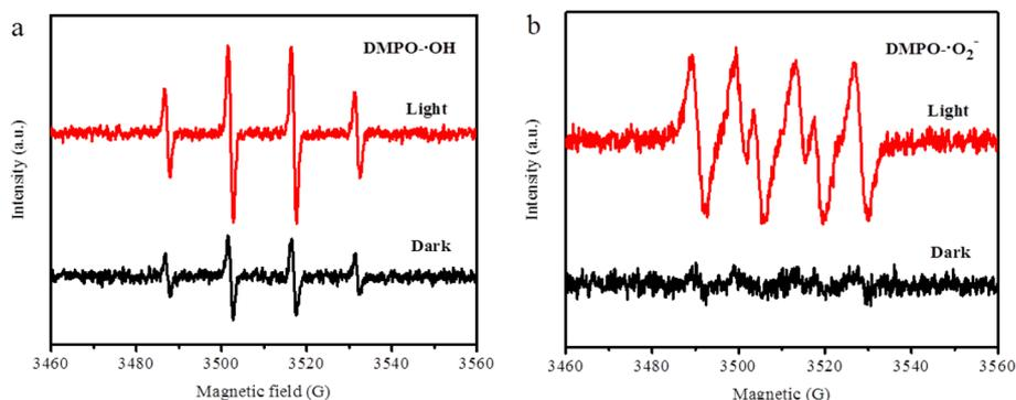
Fig. 9 ESR spectrum of CuS@Cu-CDs/H<sub>2</sub>O<sub>2</sub> system (a) DMPO- $\cdot\text{OH}$  (b) DMPO- $\cdot\text{O}_2^-$ .
